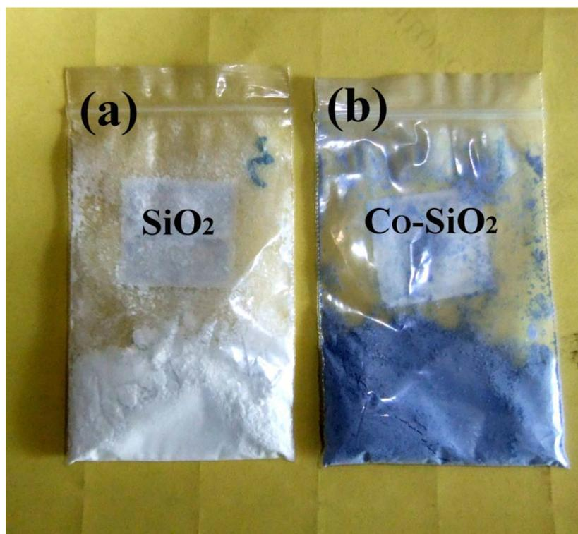
**Fig. S6** Photo of silica nanospheres prepared without (a) and with (b) adding cobalt salts.
