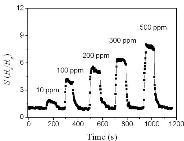
**Fig. S 14** Time-dependent response of the  $\text{Fe}_2(\text{MoO}_4)_3 @ \alpha\text{-MoO}_3$  nanorods to methanol with different concentrations at 220 °C.
