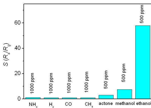
**Fig. S 13** The sensitivity of the  $\text{Fe}_2(\text{MoO}_4)_3 @ \alpha\text{-MoO}_3$  nanorods to other gases at 220 °C.
