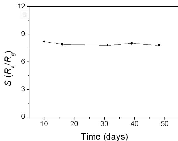
**Fig. S11** Long-term stability of the  $\text{Fe}_2(\text{MoO}_4)_3@\alpha\text{-MoO}_3$  nanorods to 100 ppm ethanol at 220 °C.
