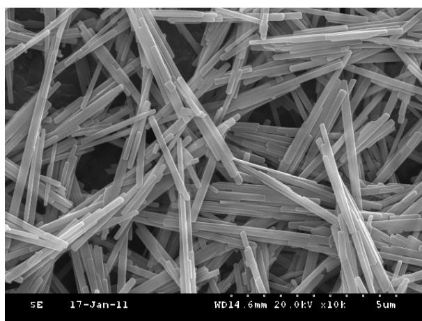
**Figure S1** A typical SEM image of the pristine α-MoO<sub>3</sub> nanorods
