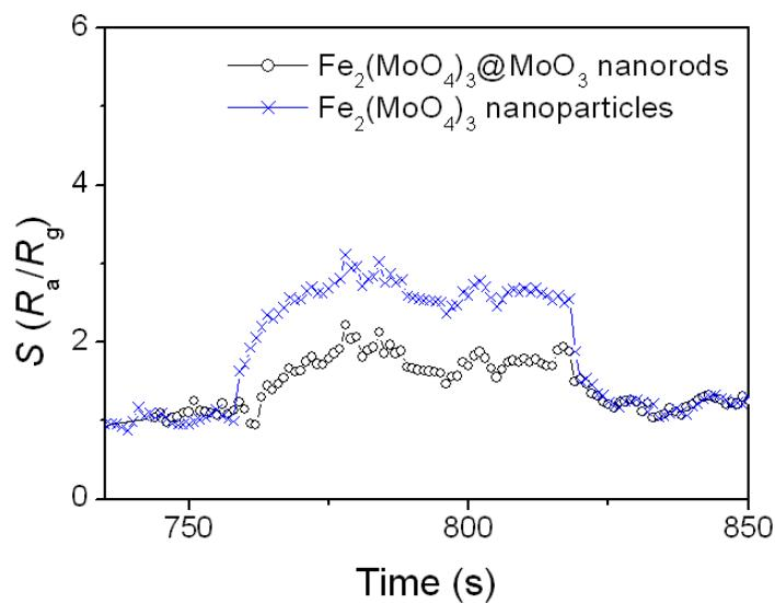
**Fig. S10** Sensor responses of  $\text{Fe}_2(\text{MoO}_4)_3@\alpha\text{-MoO}_3$  nanorods and  $\text{Fe}_2(\text{MoO}_4)_3$  nanoparticles to 10 ppm ethanol at 220 °C.
