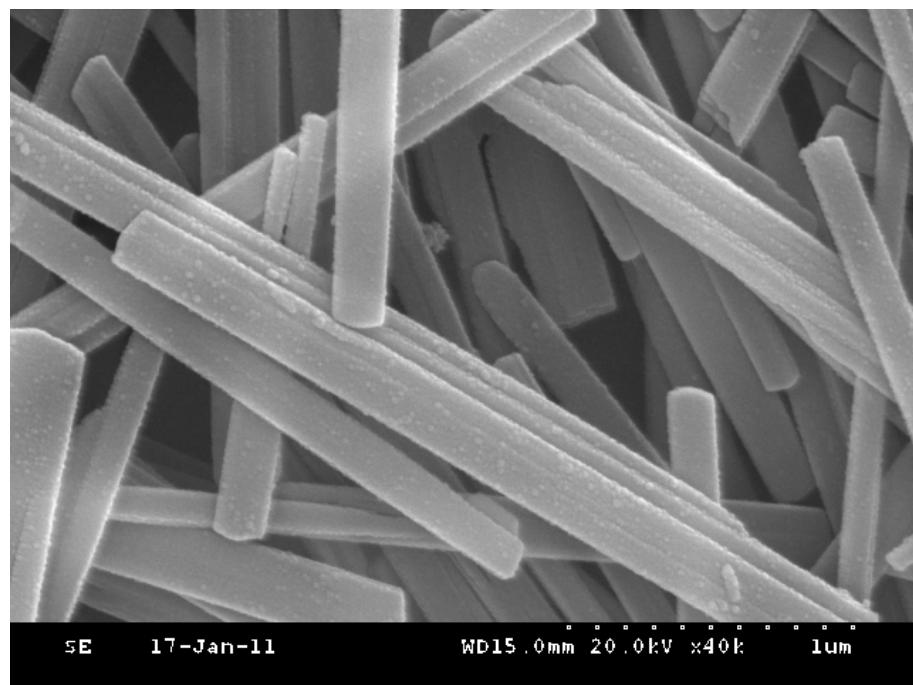
**Figure S3** A typical SEM images of Fe(OH)<sub>3</sub>@α-MoO<sub>3</sub> nanorods.
