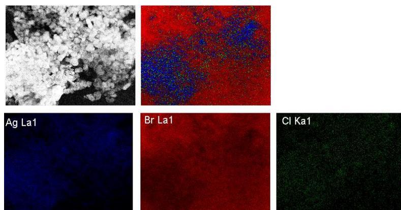
Figure S3. SEM-EDAX elemental mapping of the as-obtained AgBr/AgCl nanocashews. It is clearly showing that the sample is composed of AgBr and AgCl with cashew-like heterostructured nanoparticles.
