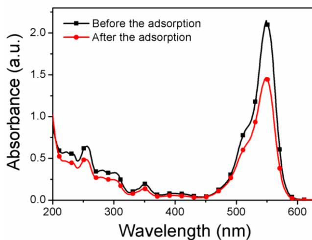
Figure S5. UV-vis spectra of RhB solution before and after adsorption on the as-prepared Ag@AgBr/AgCl nanophotocatalyst.
