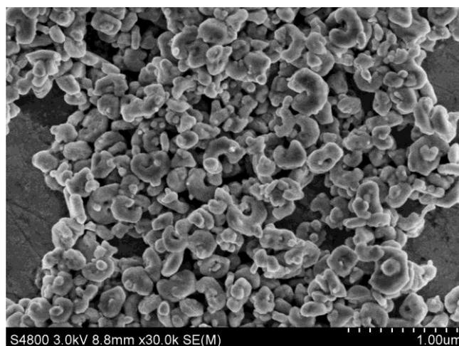
Figure S7. SEM image of Ag@AgBr/AgCl after recycling reactions.
