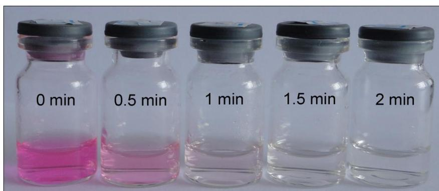
Figure S6. The color change of RhB solution with the reaction proceeds.
