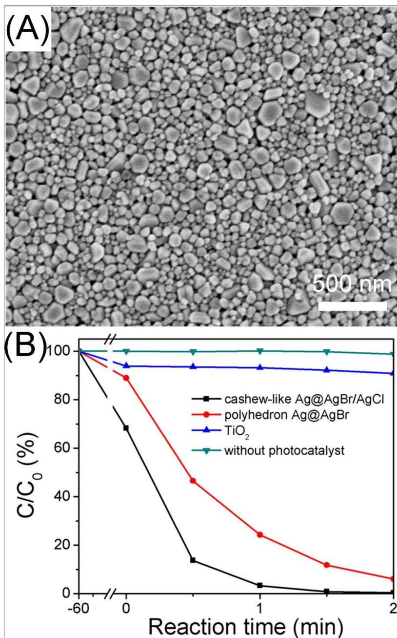
Figure S4. (A) SEM images of polyhedral Ag@AgBr; (B) The degradation curves of RhB solution with cashew-like Ag@AgBr/AgCl, polyhedron Ag@AgBr,  $TiO_2$  and without any photocatalyst under visible light irradiation.
