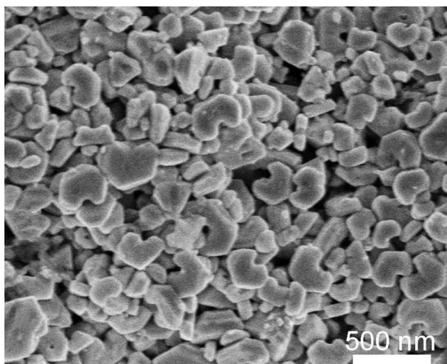
Figure S2. SEM image of the as-prepared AgBr/AgCl nanoparticles, clearly showing that the product is consisting of large amount of cashew-like nanoparticles.
