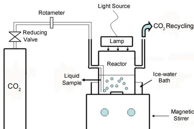
Figure S1. Schematic reaction system for photocatalytic reduction of CO<sub>2</sub>.
