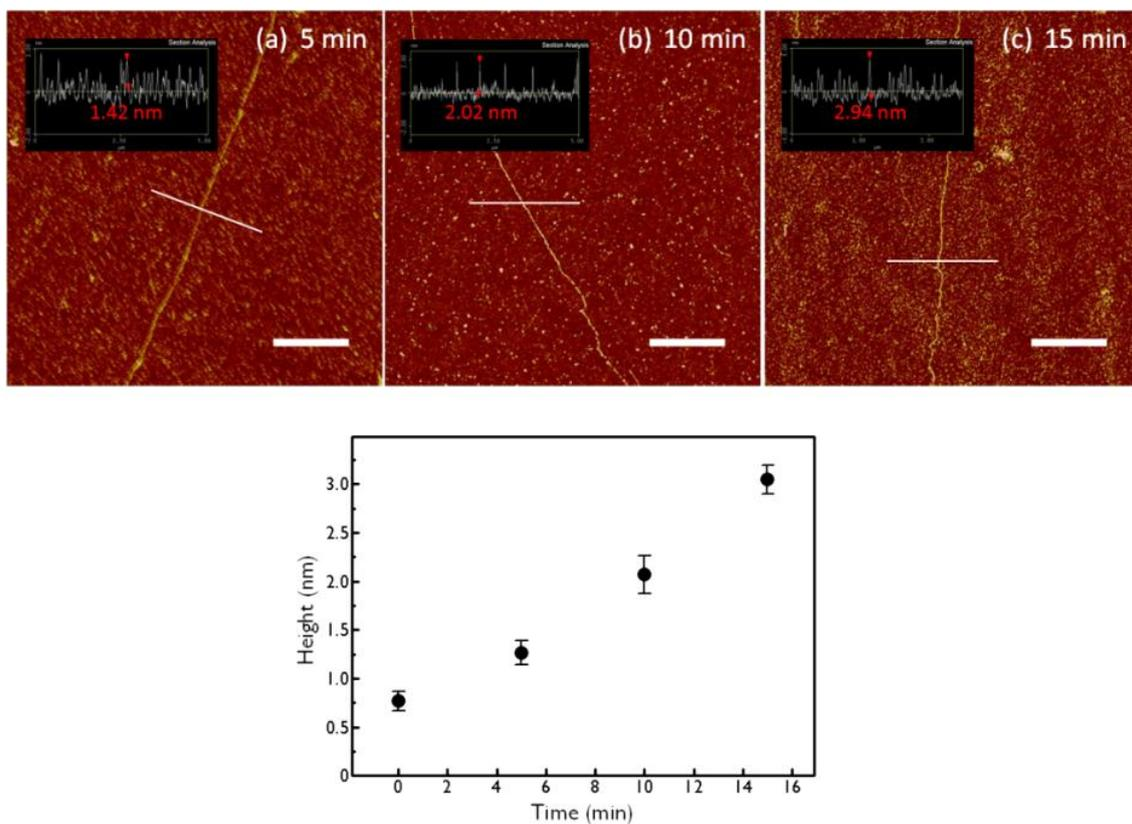
**Fig. S1** Typical AFM images of the DNA-templated polyaniline nanowires obtained by photopolymerization for 5 min (a), 10 min (b), and 15 min (c), respectively (top), and plots of the height of DNA template as a function of photopolymerization time (bottom). Image scale bar: 1.0  $\mu\text{m}$ . The height values were calculated based on AFM analyses of numerous nanowires.
