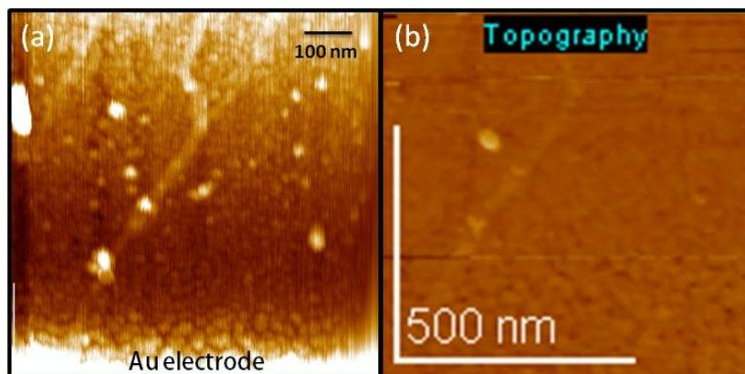
**Fig. S4** AFM images of the DNA-templated polyaniline nanowires (a) before and (b) after the PCI-AFM measurement, respectively.
