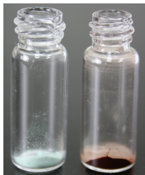
Fig. S2 MIL-101(Cr) crystals before (left) and after (right) adsorption of C70.
