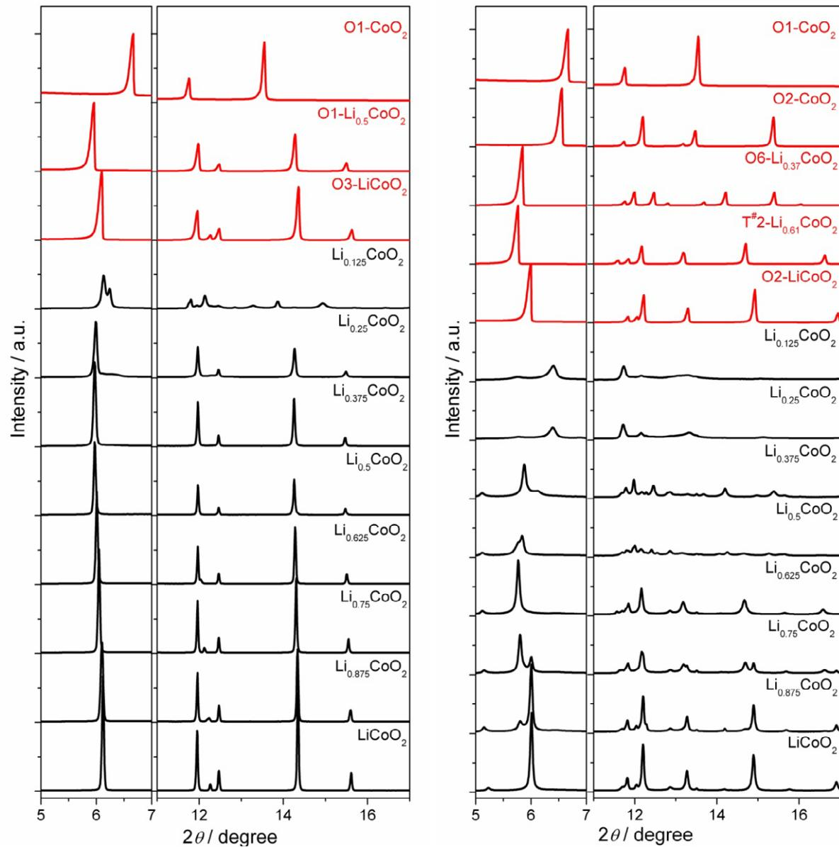
Figure S2. Synchrotron X-ray diffraction patterns of electrochemical lithium-ion de-intercalated samples of O3-LiCoO<sub>2</sub> and O2-LiCoO<sub>2</sub> drawn by black lines. The simulated patterns are also displayed by red lines.
