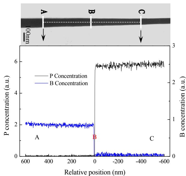
**Supporting Fig. 2** The EDS results showing the signals for B element (blue lines) and P element (black lines) along the growth direction of SnS Nanowire.
