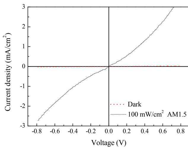
**Supporting Fig. 5** The current–voltage ( $I-V$ ) characteristics of the SnS nanowires sandwiched between ITO and Al contacts.
