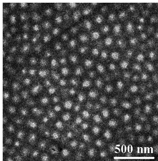
**Supporting Fig. 3** SEM image of SnS nanowire tips exposed above the photoresist layer.
