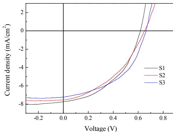
**Supporting Fig. 4** Current density vs voltage for the solar cell under simulated AM1.5G illumination with intensity of 100 mW/cm<sup>2</sup>.
