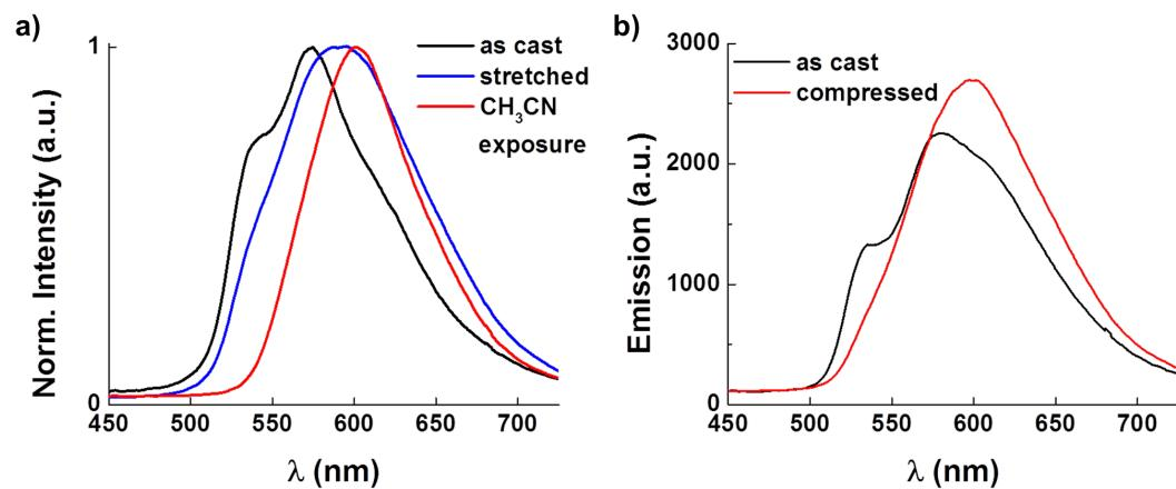
**Fig. S18.** a) Normalized emission spectra of samples of 10 wt. %  $[\text{Pt}(1\text{Cl})](\text{PF}_6)$  in PBMA film as cast and after either stretching or exposure to acetonitrile vapor, and b) unnormalized emission spectra of a 10 wt. %  $[\text{Pt}(1\text{Cl})](\text{PF}_6)$  in PEMA film before (as cast) and after compression.
