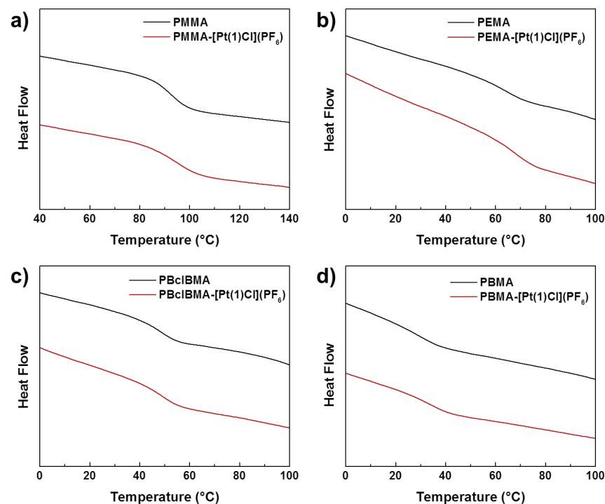
**Fig. S5.** DSC curves of the matrices and blends prepared with [Pt(1)Cl](PF<sub>6</sub>) of a) PMMA, b) PEMA, c) PBcIBMA, and d) PBMA.
