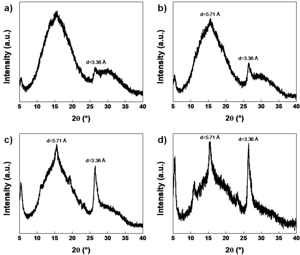
**Fig. S12.** WAXS of (a) 2.5, (b) 5, (c) 10, and (d) 20 wt. %  $[\text{Pt}(1\text{Cl})(\text{PF}_6)]$  in PMMA after compression. At 2.5 wt. % loading the scattering from the platinum complexes is mostly obscured by that of the polymer matrix. However as the loading increases peaks at  $2\theta = 15.5^\circ$  and  $26.5^\circ$  ( $d = 5.71$  and  $3.36 \text{ \AA}$  respectively) can be seen.
