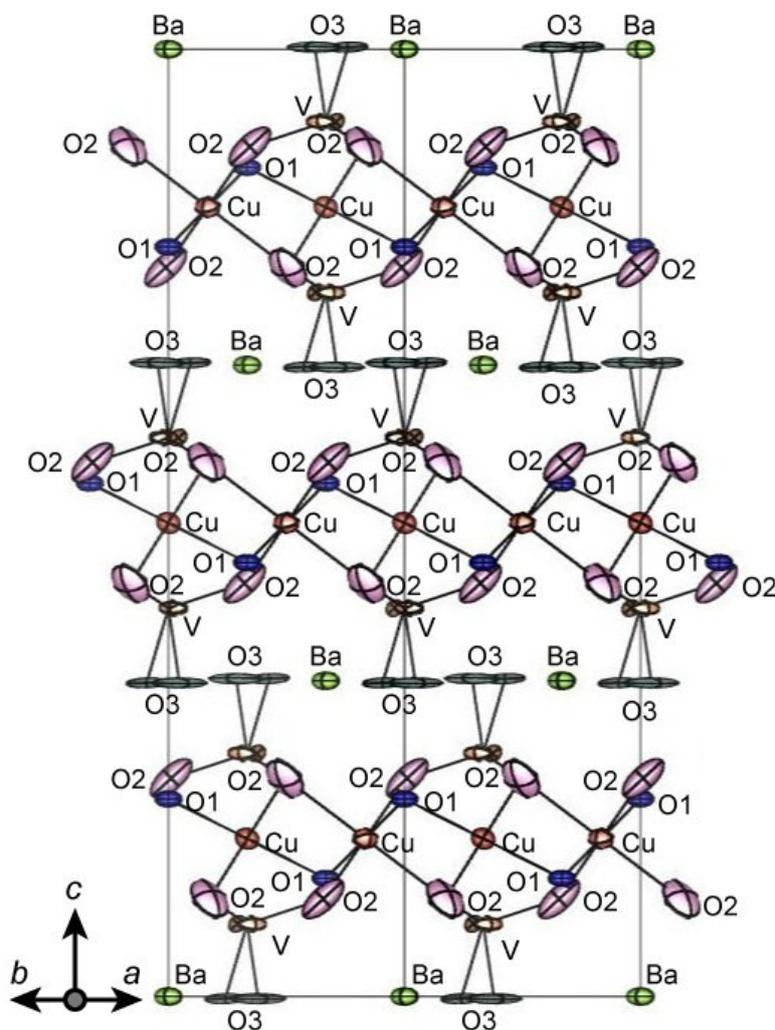
Figure S1. Crystal structure of  $\beta$ -vesignieite,  $\text{BaCu}_3\text{V}_2\text{O}_8(\text{OH})_2$  with thermal ellipsoids at 80% for legibility. The hydrogen atoms are not shown.
