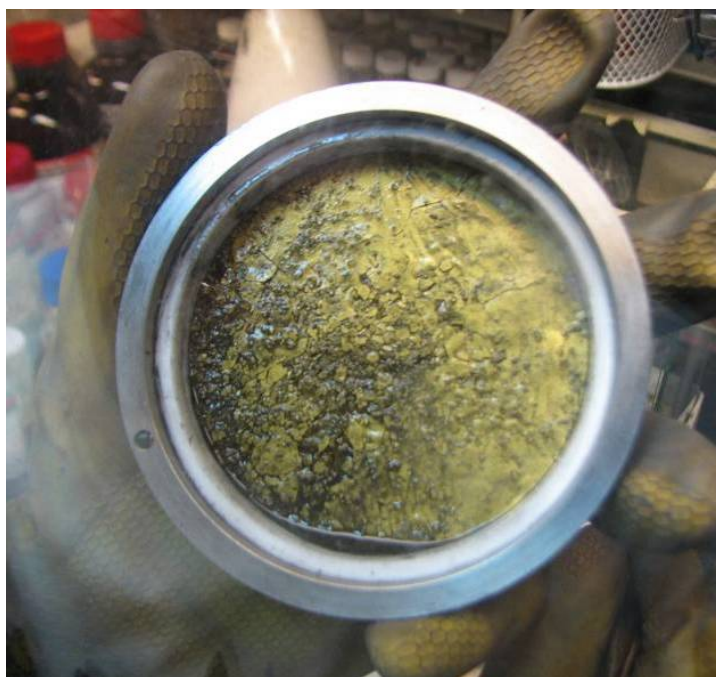
Figure S1. Photo image of Li-intercalated graphite electrode (3 inch in diameter)
