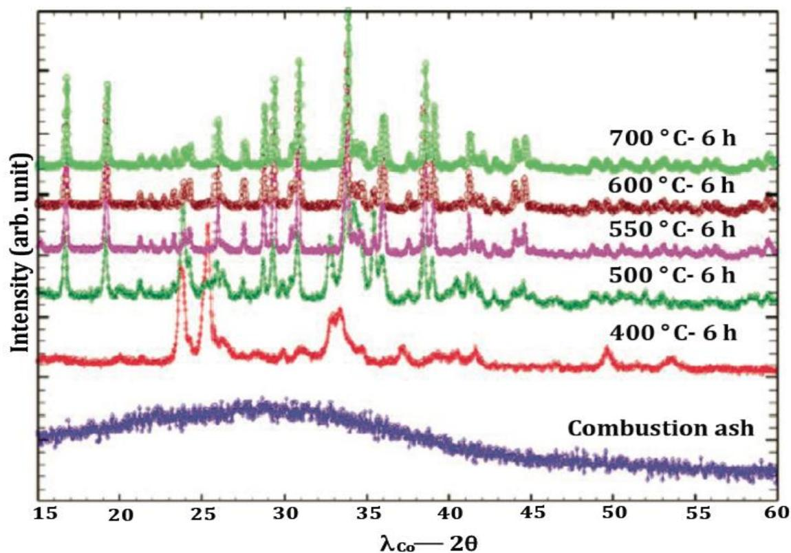
**Figure S1:** Comparative XRD patterns showing the effect of annealing temperature on the phase evolution of  $\text{Li}_2\text{FeP}_2\text{O}_7$ . The initial combustion ash shows a broad XRD profile owing to amorphous intermediate complex. High-temperature treatment slowly transforms this complex to form the final product. Single-phase product was obtained at 550°C onwards.
