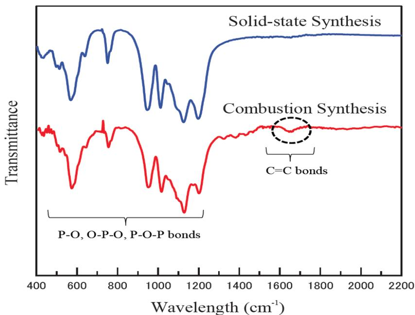
**Figure S2:** Comparative FT-IR spectra of  $\text{Li}_2\text{FeP}_2\text{O}_7$  made by conventional solid-state synthesis and solvothermal (combustion) synthesis. While in P–O–P, O–P–O and P–O bands are common to both sample, the combustion synthesized sample show an extra prominent band at  $1600\text{ cm}^{-1}$ , proving the presence of graphitic carbon coating of the pyrophosphate sample.
