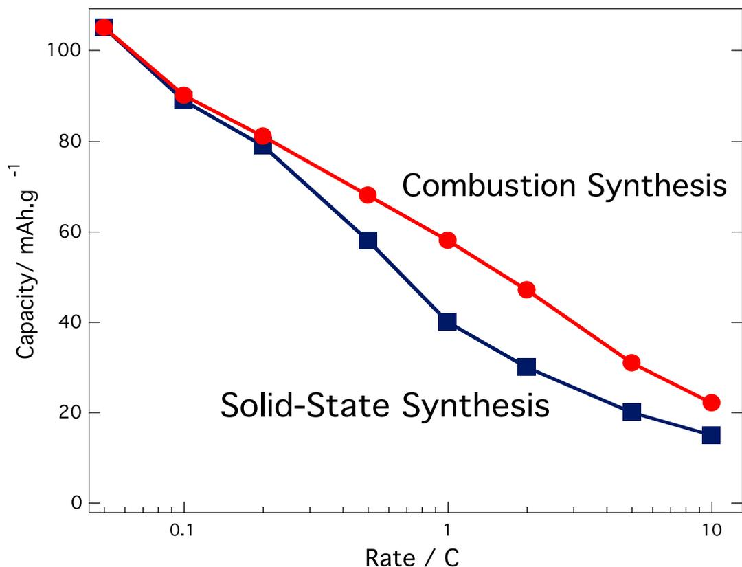
**Figure S4:** Power rate capability of splash combustion synthesized  $\text{Li}_2\text{FeP}_2\text{O}_7$  vs solid-state synthesized  $\text{Li}_2\text{FeP}_2\text{O}_7$ . Though combustion synthesized (nanometric) product gives slightly better capacity at faster rate, the overall capacity is quite independent of particle size owing to its two-dimensional diffusion channels.
