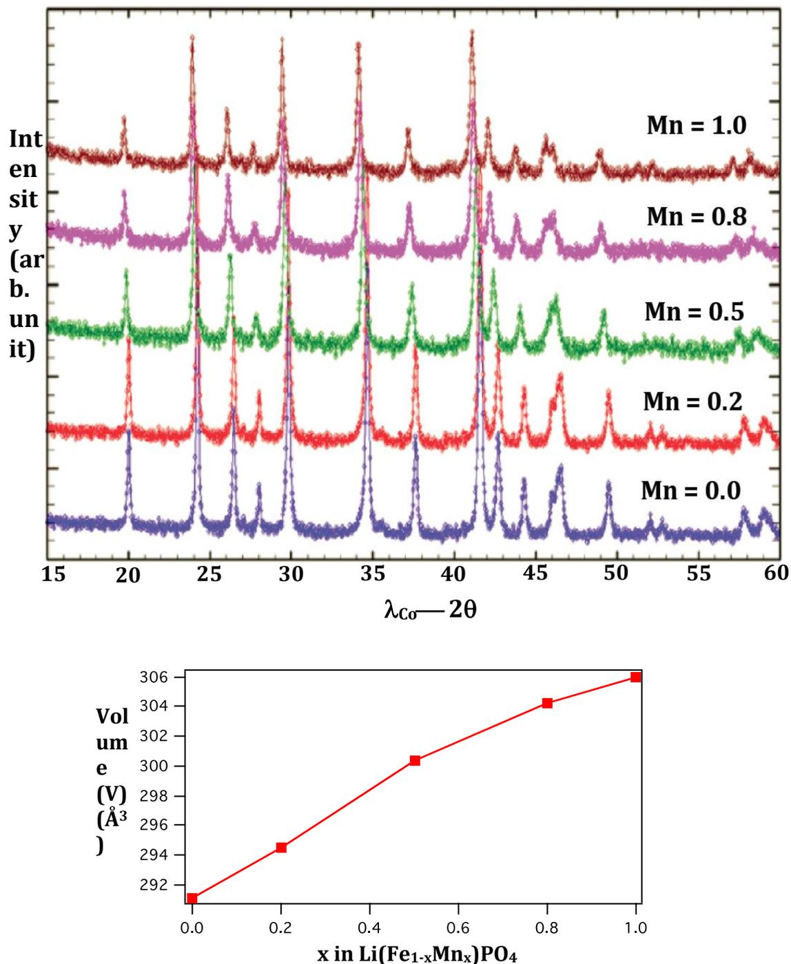
**Figure S8:** (Top) Combustion synthesized mixed-metal  $\text{Li}(\text{Fe}_{1-x}\text{Mn}_x)\text{PO}_4$  olivine ( $x = 0, 0.2, 0.5, 0.8$  and  $1$ ), showing gradual up shift in the XRD peaks with higher Mn-content owing to its larger ionic radii. These phases were produced at  $300\text{ }^\circ\text{C}$  for  $1\text{ h}$ . (Bottom) The gradual increase in lattice volume with Mn content is shown.
