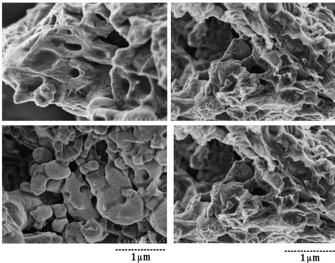
**Figure S3:** Representative SEM micrographs showing the porous morphology of combustion synthesized  $\text{Li}_2\text{FeP}_2\text{O}_7$  particles. The continuous evolution of gaseous products leads to this porous morphology.
