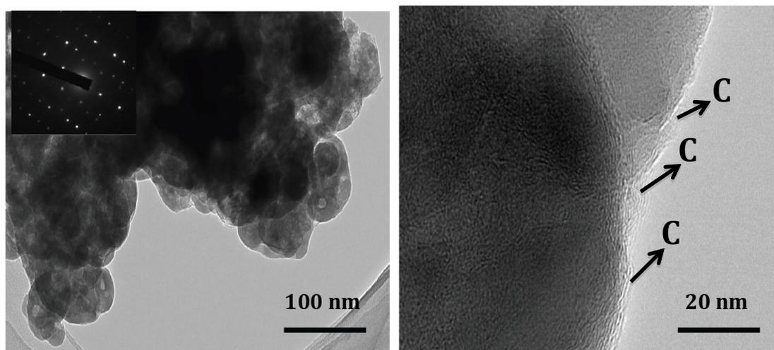
**Figure S7:** (Left) HRTEM images of combustion synthesized  $\text{LiFePO}_4$  showing fine particles below 100 nm. (Right) TEM observation of the formation of a thin (3-5 nm) layer of carbon coating on the individual  $\text{LiFePO}_4$  particles (as pointed by arrow marks). Thus, combustion synthesis can facilitate both 'nano-sizing' and 'carbon coating', two essential points to develop electroactive olivine cathode.
