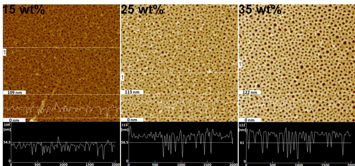
Figure SI1. 20 x 20  $\mu\text{m}$  AFM images of the nanostructures obtained with 15, 25 and 35 PS wt% and their corresponding cross-section profiles.
