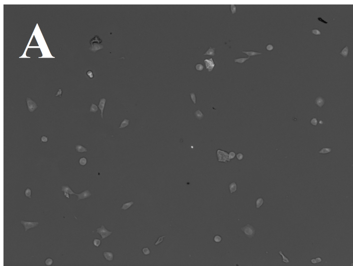
Figure S15. The photographs of the cell adhesion assay observed after 3T3 fibroblast cell culturing for 4 hrs at 37 °C by inverted fluorescence microscopy on the bare (A), PEAC-modified (B) and further thiol (MPA) modified (C) substrate surfaces of glass. All the figures have the same scale bar as in Figure 5 in the main text.
