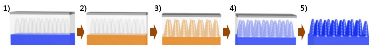
Figure S1. Schematic diagram of the vacuum-assisted template wetting method for the fabrication of P-ARSs on a PMMA film surface. 1) The PMMA film was deposited on an AAO template with nanopores on one surface and placed in a vacuum. 2) The entire set was heated to a temperature higher than the glass transition temperature of PMMA. 3) The heated PMMA film was pressed against the AAO template to seal the nanopores, and the vacuum was released so that the nanopores in AAO could be filled with molten PMMA as a result of the difference in surface tension between the alumina wall and polymer; this process was facilitated by the difference in pressure between inside and outside the pores. 4) When the pores were filled completely, the entire set was cooled to room temperature. 5) The AAO template was dissolved chemically so that the PMMA film contained P-ARSs on a single surface.
