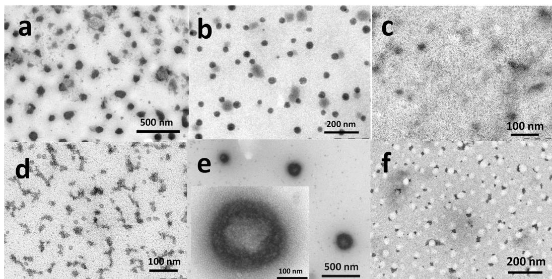
**Fig. S9.** TEM images (a, b, c) of the formed aggregates and micelles before the addition of formaldehyde, and TEM images (d, e, f) of the formed aggregates and micelles after 1 min of the formaldehyde was added, with different ethanol/water volume ratios: (a, d) 4/24, (b, e) 8/20, and (c, f) 12/16.
