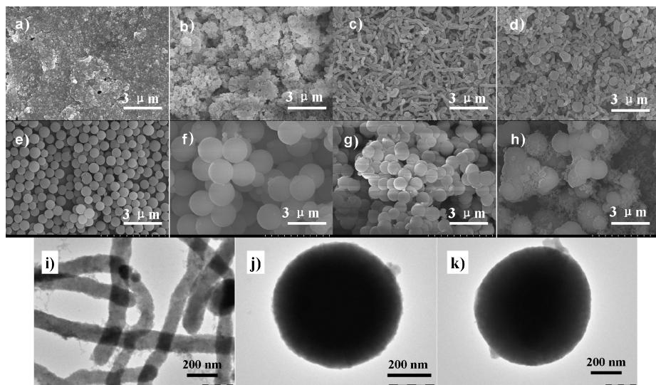
**Fig. S1.** SEM images (a-g) and TEM images (i-k) of the PSS composites prepared with different ethanol/water volume ratios: ethanol/water volume ratio = 0:28 (a); 2/26 (b); 4/24 (c, i); 6/22 (d); 8/20 (e, j); 10/18 (f); 12/16 (g, k); 14/10 (h).
