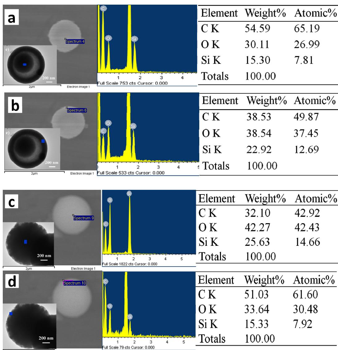
**Fig. S4.** EDX spectra and the element composition of the core and shell of the CS composites (a,b: E8-CS, b,c: E12-CS).
