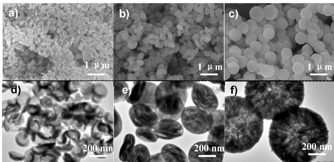
**Fig. S8.** SEM images (a-c) and TEM images (d-f) of the silica products without the addition of formaldehyde. The ethanol/water volume ratios were 4/24 (a,d), 8/20 (b,e), and 12/16 (c,f).
