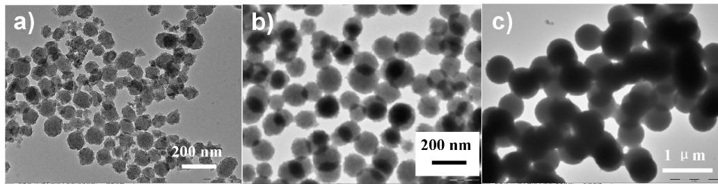
**Fig. S6.** TEM images of the mesoporous silica spheres prepared without the addition of RF precursor. The ethanol/water volume ratios were 4/24 (a), 8/20 (b), and 12/16 (c).
