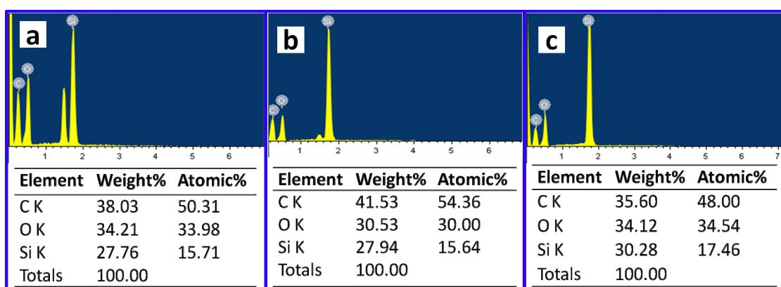
Figure S2. EDX spectra and the element composition of CS composites (a: E4-CS, b: E8-CS, c: E12-CS).
