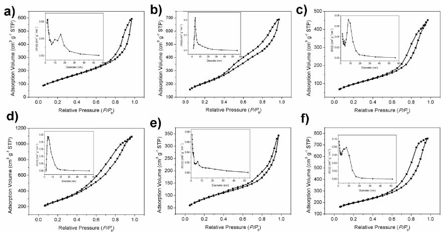
**Fig. S5.** N<sub>2</sub> sorption isotherms and pore size distributions (inset) of the samples prepared with different ethanol/water volume ratios: (a) E4-SiO<sub>2</sub>; (b) E4-C; (c) E8-SiO<sub>2</sub>; (d) E8-C; (e) E12-SiO<sub>2</sub>; (f) E12-C.
