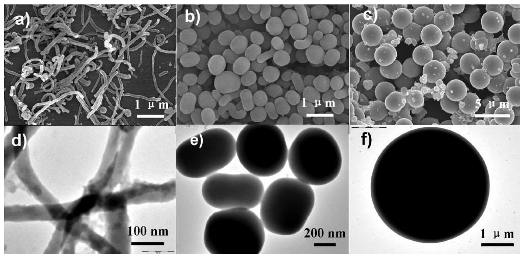
**Fig. S7.** SEM images (a-c) and TEM images (d-f) of the RF polymer products without the addition of TEOS. The ethanol/water volume ratios were 4/24 (a,d), 8/20 (b,e), and 12/16 (c,f).
