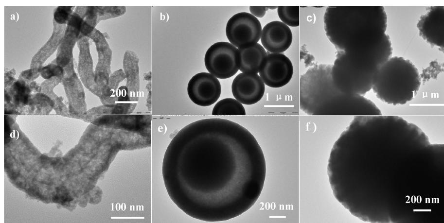
**Fig. S3.** TEM images of the carbon-silica (CS) samples E4-CS (a,d), E8-CS (b,e), and E12-CS (c,f).
