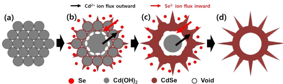
**Scheme S2.** Schematic diagram of the entire process via Kirkendall diffusion effect. The interdiffusion of  $\text{Se}^{2-}$  and  $\text{Cd}^{2+}$  occurs through the CdSe outer shell.
