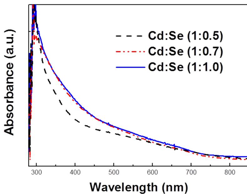
**Figure S2.** UV-vis absorption spectra compared with atomic ratios of the prepared thorny CdSe nanotubes.
