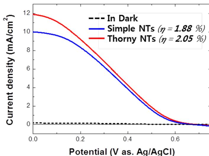
Figure S3.  $I$ - $V$  characteristics of PEC solar cell using a photoanode compared of simple nanotubes (Simple NTs) and hierarchical thorny nanotubes (Thorny NTs) of CdSe.
