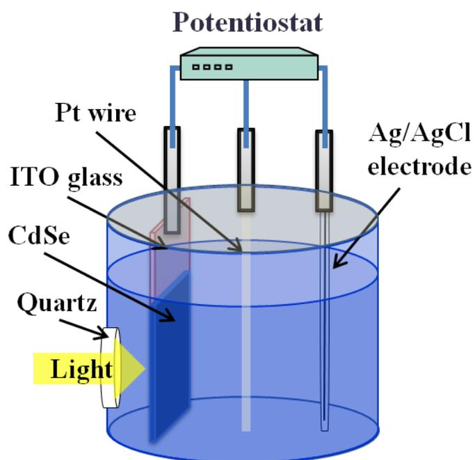
**Scheme S1.** Schematic diagram illustrating the fabrication of photoelectrochemical cell by using three-electrode configuration (ITO/CdSe nanostructure/poly sulfide electrolyte/Pt)
