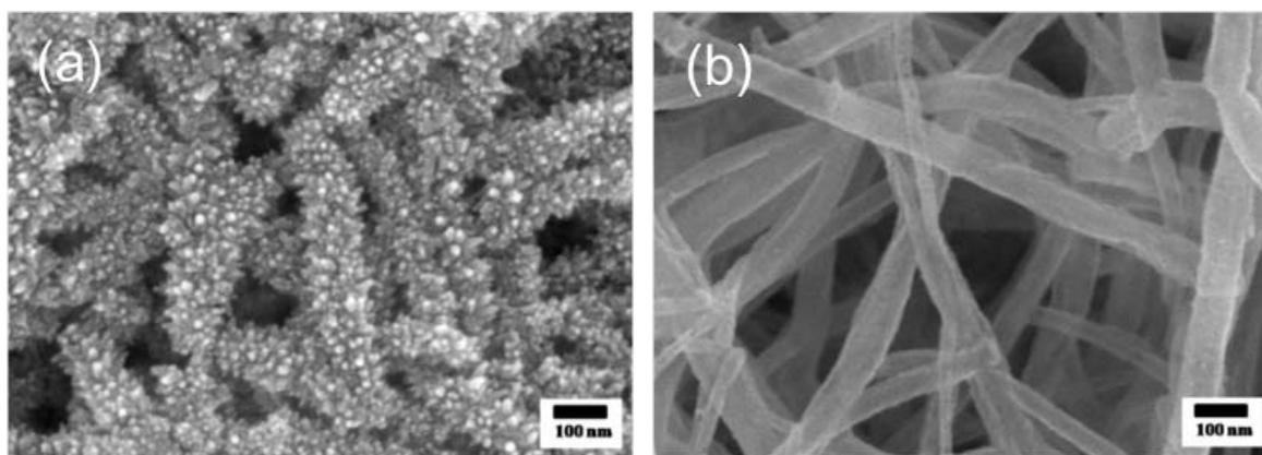
**Figure S1.** The surface morphology of (a) hierarchical thorny CdSe nanotubes and (b) CdSe nanotubes
