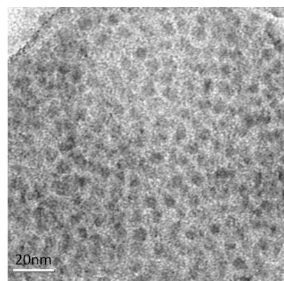
**Fig. S2.** TEM image of FePt NPs prepared by Fr-biomimetic synthesis.
