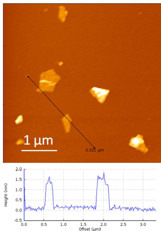
**Fig. S1.** AFM height image of GN-PNHS and section analysis.
