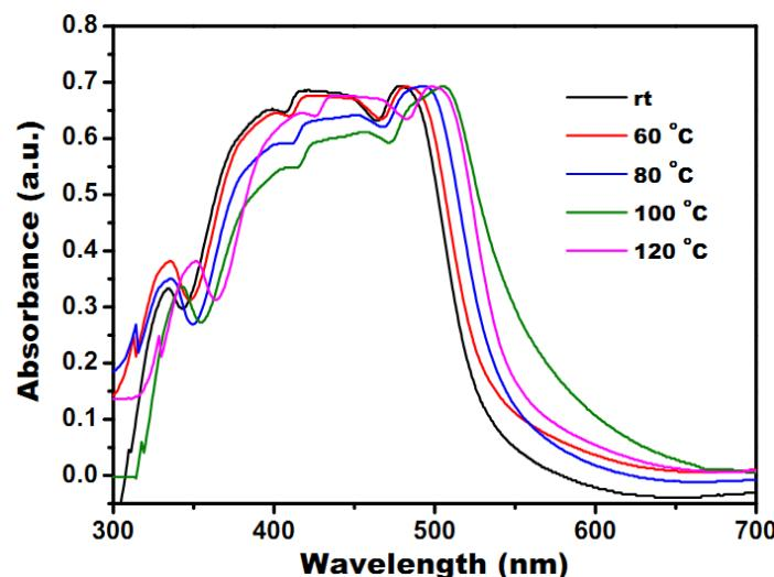
**Figure S1.** UV-vis absorption spectra of **DPPAIT** thin films of different annealing temperatures on ITO substrate
