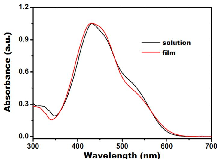
**Figure S2.** UV-vis absorption spectra of THF solution and the solid thin film of **DPAPPD**.
