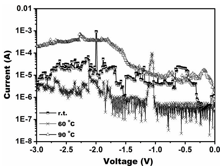
**Figure S5.** I-V characteristics of the memory devices fabricated with **DPAPPD** films annealed at different temperatures.
