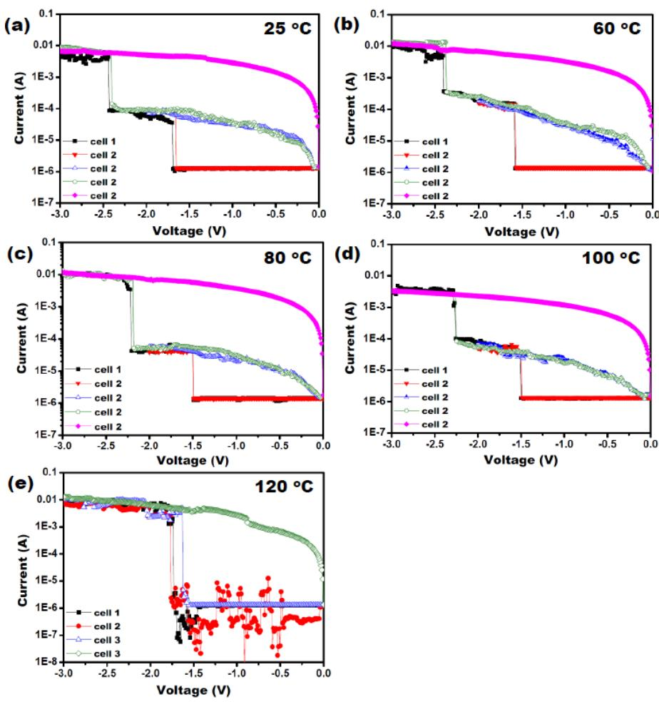
**Figure S6.**  $I$ - $V$  characteristics of the memory device fabricated with **DPAPIT** annealed at different temperatures: a) without annealing, b) 60 °C, c) 80 °C, d) 100 °C, e) 120 °C, respectively.
