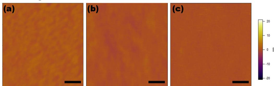
**Figure S3.** Tapping-mode AFM image of **DPAPPD** thin films deposited onto ITO substrate of different annealing temperatures: (a) without annealing, (b) 60 °C, and (c) 90 °C. The color bar of the three images were displayed in the right of (c). The scale bar corresponds to 1 μm.
