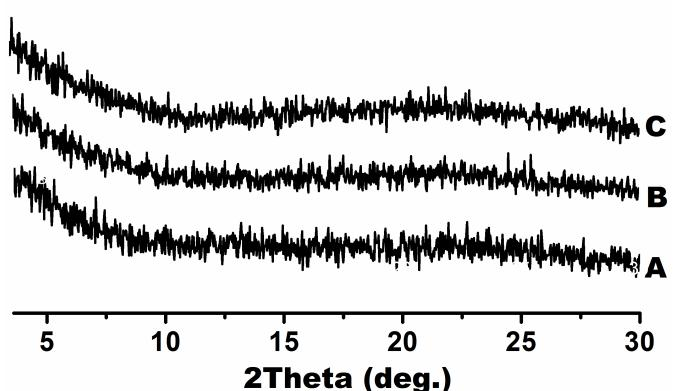
**Figure S4.** XRD pattern of **DPAPPD** films annealed at different temperatures: A) without annealing, B) 60 °C, and C) 90 °C.
