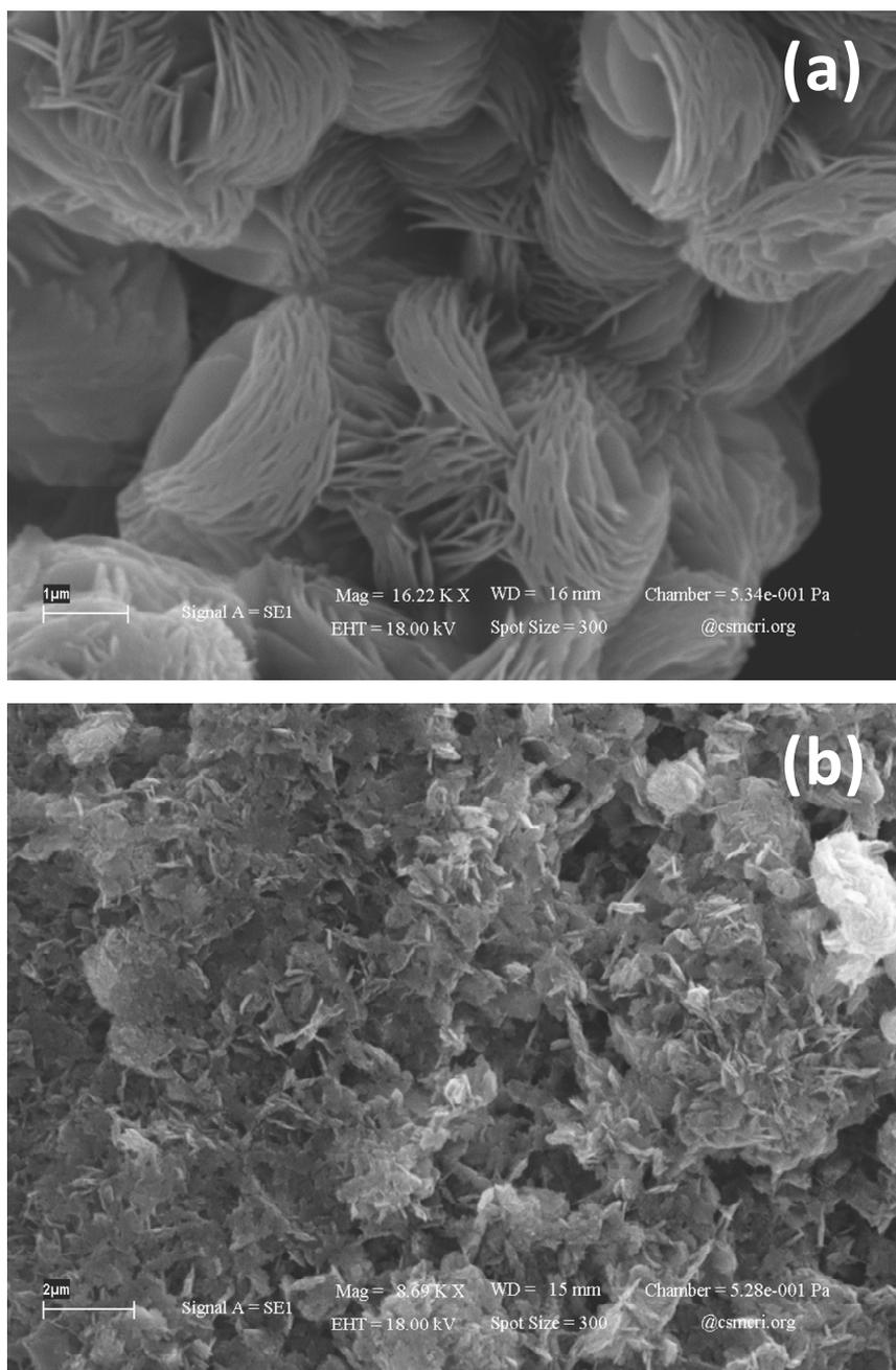
**Fig. S3.** SEM image of the hydrozincite after 8 h (a) and 20 h (b) of stirring at room temperature using 10 g ammonium carbonate for 4 g bulk ZnO.
