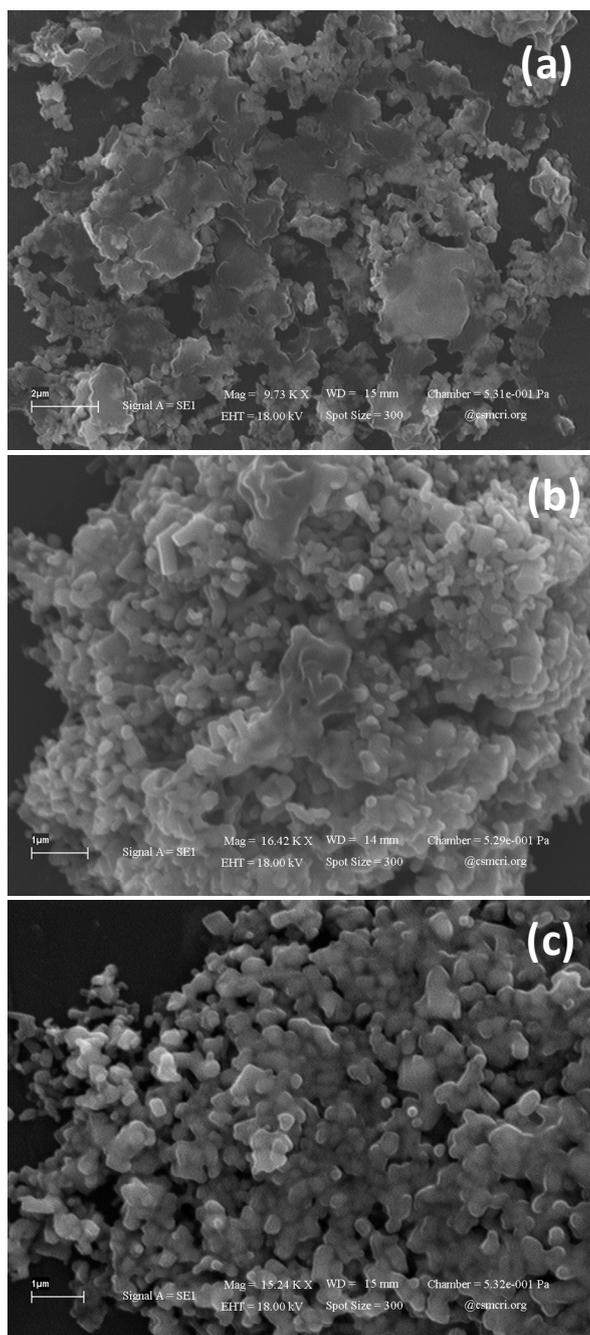
**Fig. S4.** SEM image of the hydrozincite after 30 min in the control reactions using (a) sodium carbonate, (b) sodium hydroxide and (c) ammonium hydroxide instead of ammonium carbonate.
