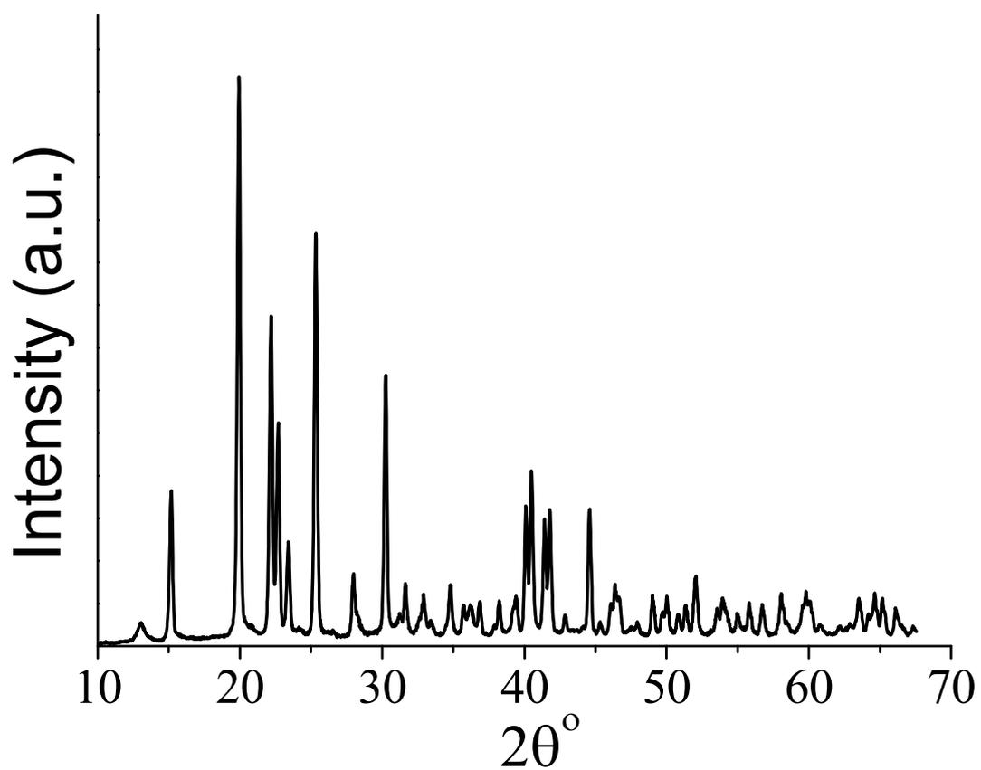
**Fig. S5.** X-ray diffraction pattern of intermediate obtained after 5 min for the of reaction at room temperature using 10 g ammonium carbonate for 4 g bulk ZnO.
