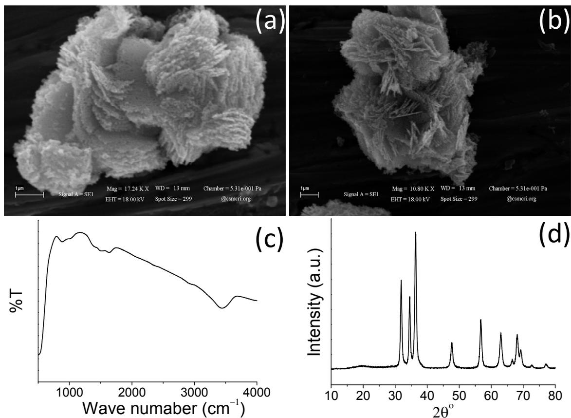
**Fig. S5.** Re-generated hierarchically assembled porous ZnO nanoflakes after 4<sup>th</sup> cycle (a & b) SEM image (c) FT-IR spectrum, and (d) X-ray diffraction pattern and.
