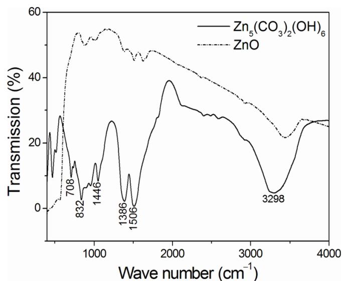
**Fig. S2.** FT-IR spectra of (a) hydrozincite intermediate and (b) the corresponding porous ZnO obtained after calcination at 500°C for 5 h.
