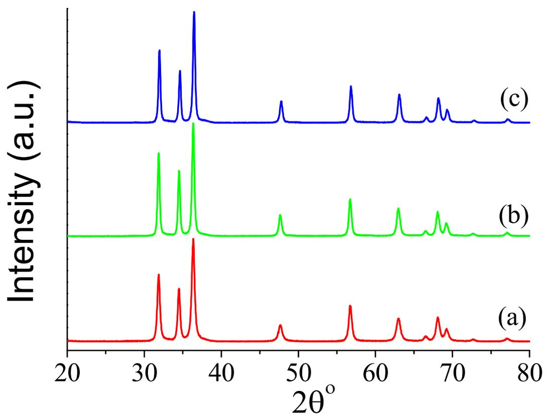
**Fig. S1.** X-ray diffraction pattern of the hierarchically assembled porous ZnO nanoflakes after calcination at 450 °C (a), 500 °C (b) and 600 °C (c).
