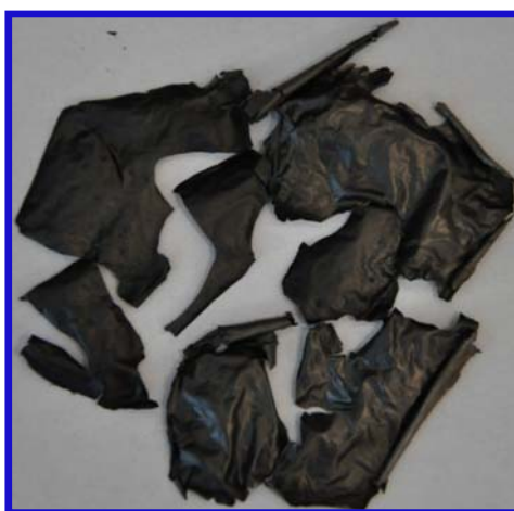
Fig. S2 A digital optical image of vacuum filtration derived free-standing CNT films rolled up and folded.
