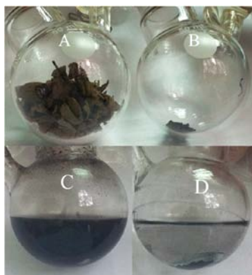
Figure S9. Photos of GO (A) and active carbon (B) in round flask. Photos of reaction mixture in round flask with GO (C) and active carbon (D) after deodorization.
