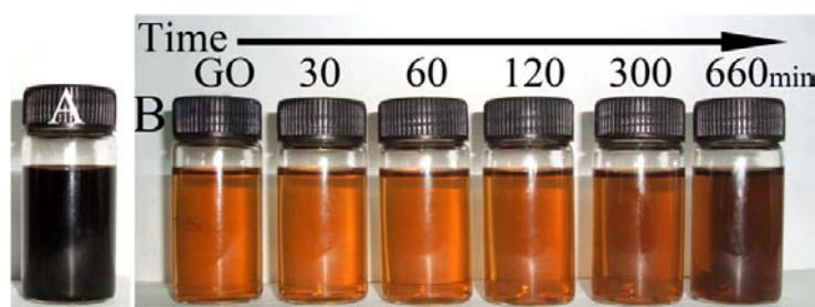
Figure S1. Photos of GO dispersion from control reaction at 80 °C in water in the absence of mercaptan. (A) Original reaction dispersion after heating for 660 min in water; (B) DMF-diluted GO dispersion at different reaction time.
