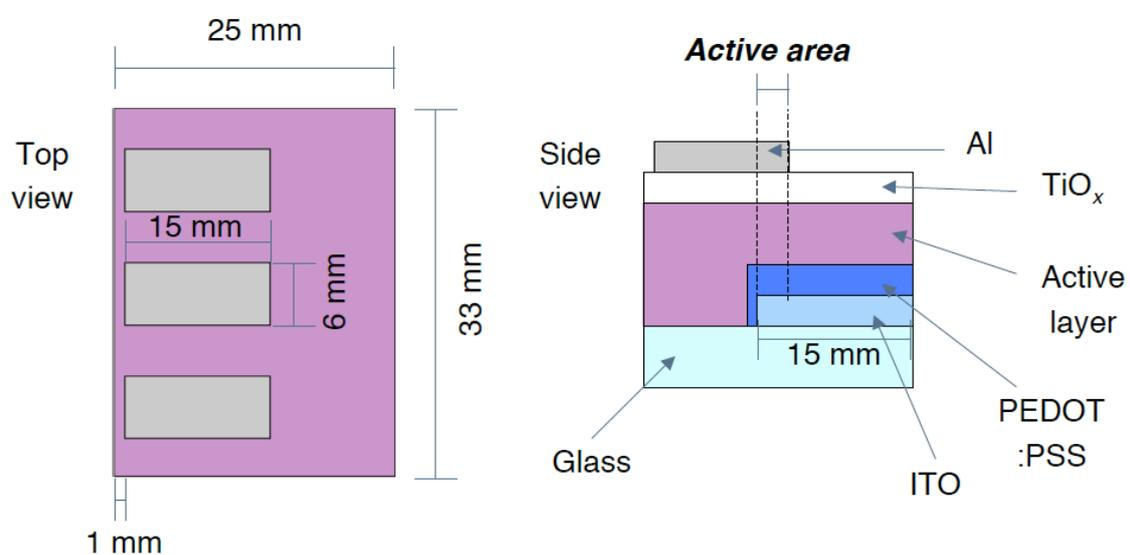
**Fig. S3** Schematic illustrations of top and side views of the ITO/PEDOT:PSS/polymer:PCBM/TiO<sub>x</sub>/Al device.
