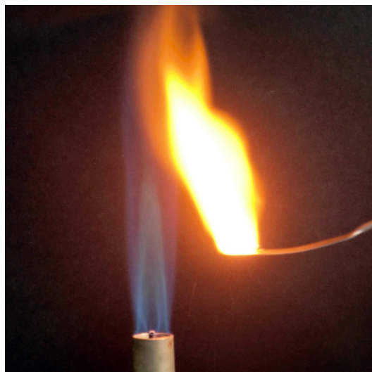
Figure S6 TKX-50 held in the flame on a spatula burns without detonation.
