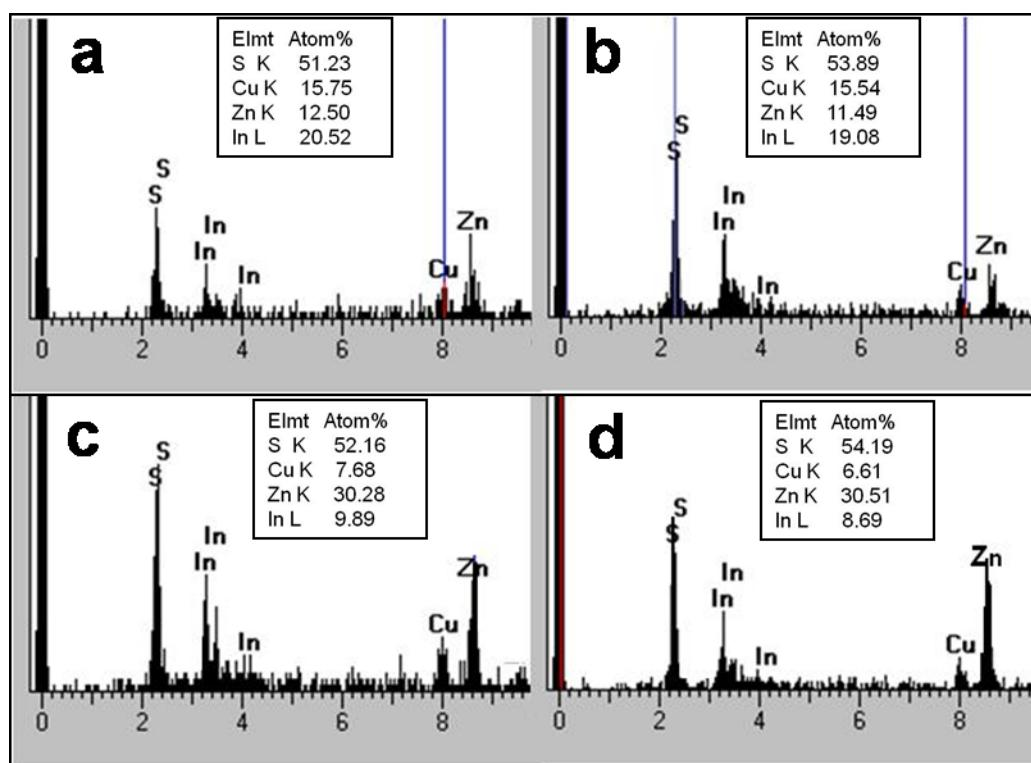
**Figure S1.** EDX spectra of  $\text{CuInZn}_x\text{S}_{2+x}$  ( $x=0.6$ ) cores (a-b) and  $\text{CuInZn}_x\text{S}_{2+x}/\text{ZnS}$  core/shell nanocrystals (c-d).
