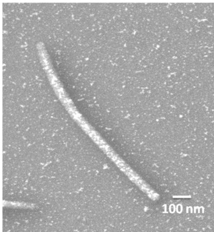
**Figure 6S:** SEM image of gold/polymer hybrid nanofibres obtained using the *ex-situ* approach where the polymer nanofibres were cross-linked with UV before exposing it to Au nanoparticle dispersion.
