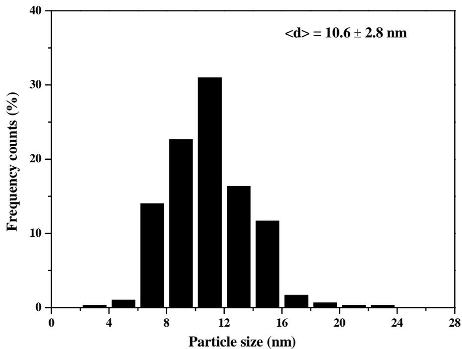
**Figure 7S:** Size-distribution histogram of gold nanoparticles prepared using the in-situ approach on the P4VP hairy shell of the PS nanofibres (corresponding to TEM image shown in Figure 5 of the manuscript).
