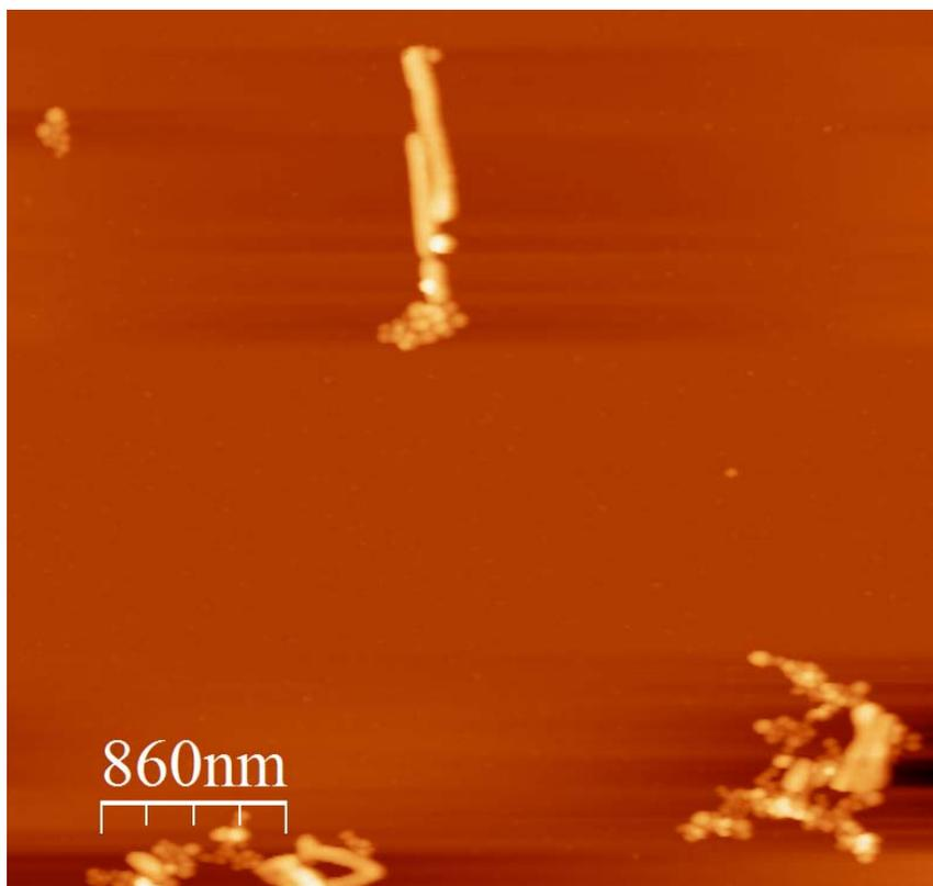
**Figure 8S:** AFM topography image of spin-coated polymer nanofibres on the silicon wafer. The sample was prepared from the methanol dispersion of PS-*b*-P4VP copolymer aged for more than four weeks. The image clearly shows the presence of spherical structures apart from nanofibres which suggest that the nanofibres formed spherical micelles when kept in methanol for long time.
