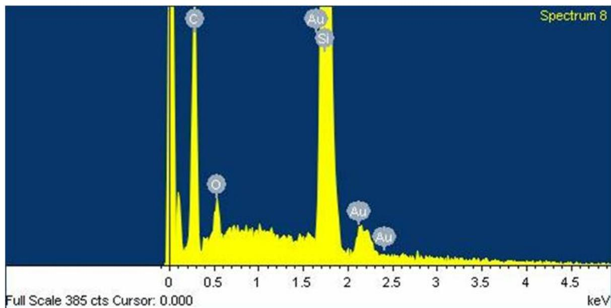
**Figure 5S:** EDX spectra of gold-polymer hybrid nanorods obtained from the sample where gold salt was first coordinated with the P4VP chains in the solution before depositing the polymer nanofibres on the substrate. The EDX spectra clearly show the presence of Au on the nanofibres.
