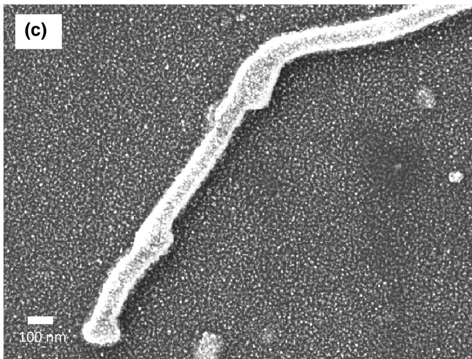
**Figure 4S:** SEM images of gold/polymer hybrid nanofibres prepared using ex-situ approach and obtained after different exposure time of the nanofibres to the Au nanoparticle dispersion a) 1 min; b) 10 min; c) 2 hours
