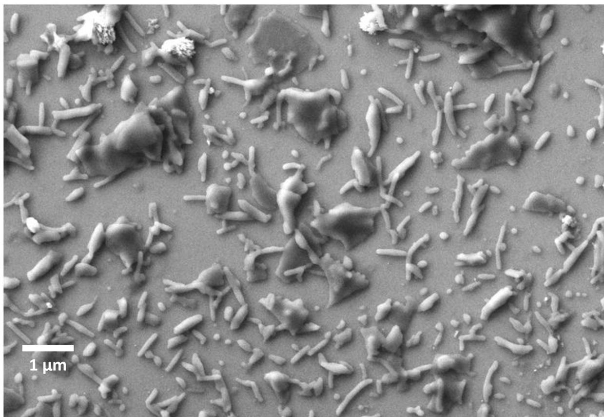
**Figure 2S:** SEM image of polymer nanofibres immobilized on the silicon wafer obtained by drop casting.
