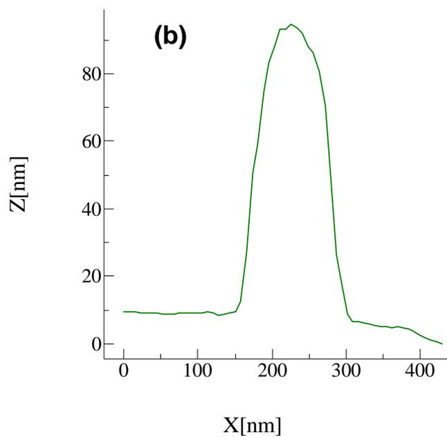
**Figure 3S:** AFM topography image of spin-coated polymer nanofibres prepared from PS-*b*-P4VP on the silicon wafer a) Height image and (b) corresponding cross-sectional profile of the nanofibre across the line marked on (a).
