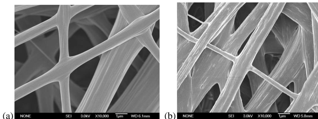
**Fig. S3** SEM images of the electrospun film fibers before (a) and after (b) PVP was removed.
