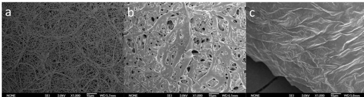
**Fig. S1** SEM images of the electrospun film from the thermoplastic SMP in cycles of shape memory test. a) the as prepared film; b) film after the first cycle of the shape memory test; c) film after the third cycle of shape memory test.
