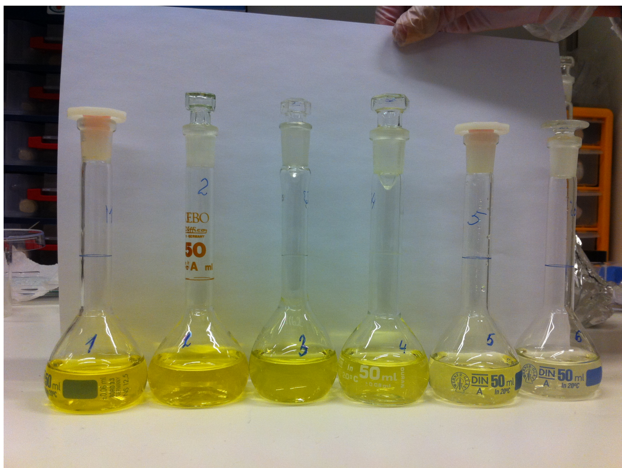
Figure FS9 Calibration curve and reference solutions for spectrophotometric determination of dichromate ion, \text{Cr}_2\text{O}_7^{2-} , adsorption capacity.
