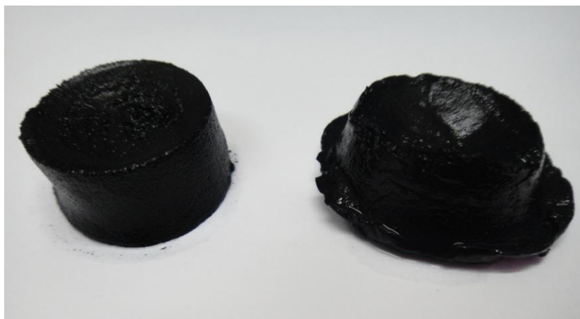
Fig. S10 Photograph of GSs prepared with 0.5 g (left one) and 0.7 g (right one) thiourea.
