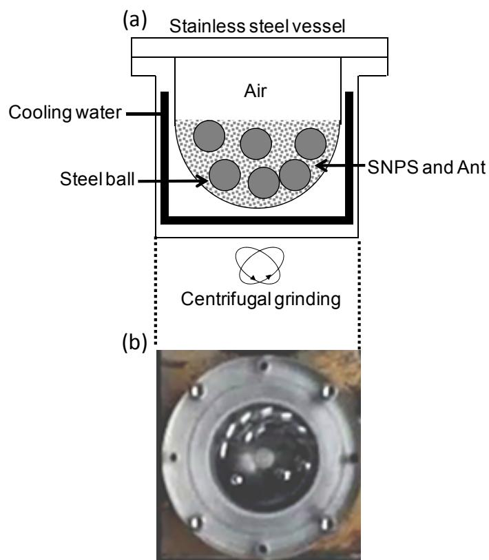
**Fig. S1.** (a) Set-up for the mechanochemical reaction, and (b) photograph of the top view of the equipment during the milling. The vessel made from a stainless steel rod (SUS304) with the inner volume of 70 mL was surrounded by a water jacket.
