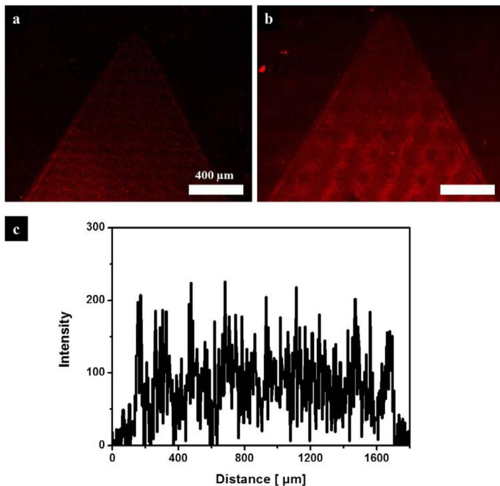
**Figure S6.** Comparison between the confocal microscope images measured for R6G adsorbed on metallic nanotip arrays (a) without and (b) with nanoscale roughness at the same experimental conditions. (c) Fluorescent intensity derived from R6G-adsorbed dual length-scale nanotip arrays under 15 min He-Ne laser irradiation.
