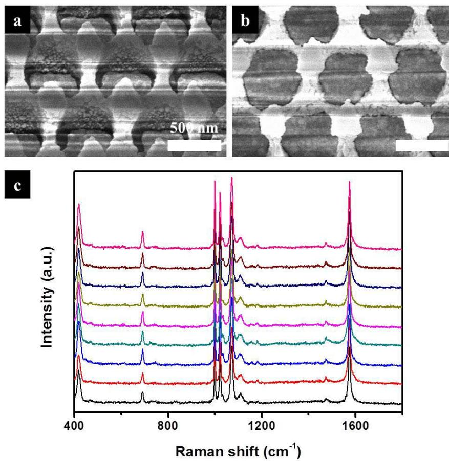
**Figure S4.** (a) 30° tilted, and (b) top view SEM images of the resulting triangular pyramid-shaped nanotip arrays after the directional Ag (25 nm)-deposition step using 3 min-etched 2-layer FCC structures, respectively. (c) SERS spectra of BT obtained from nine randomly selected spots on the triangular pyramid-shaped nanotip arrays. The laser power on samples was 75 mW, and data acquisition involved 5 sec accumulation.
