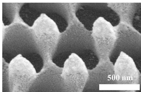
**Figure S5.** 30° tilted SEM image of the triangular pyramid-shaped nanotip arrays without nanoroughness, after the isotropic Ag thin film (10 nm)-deposition step.
