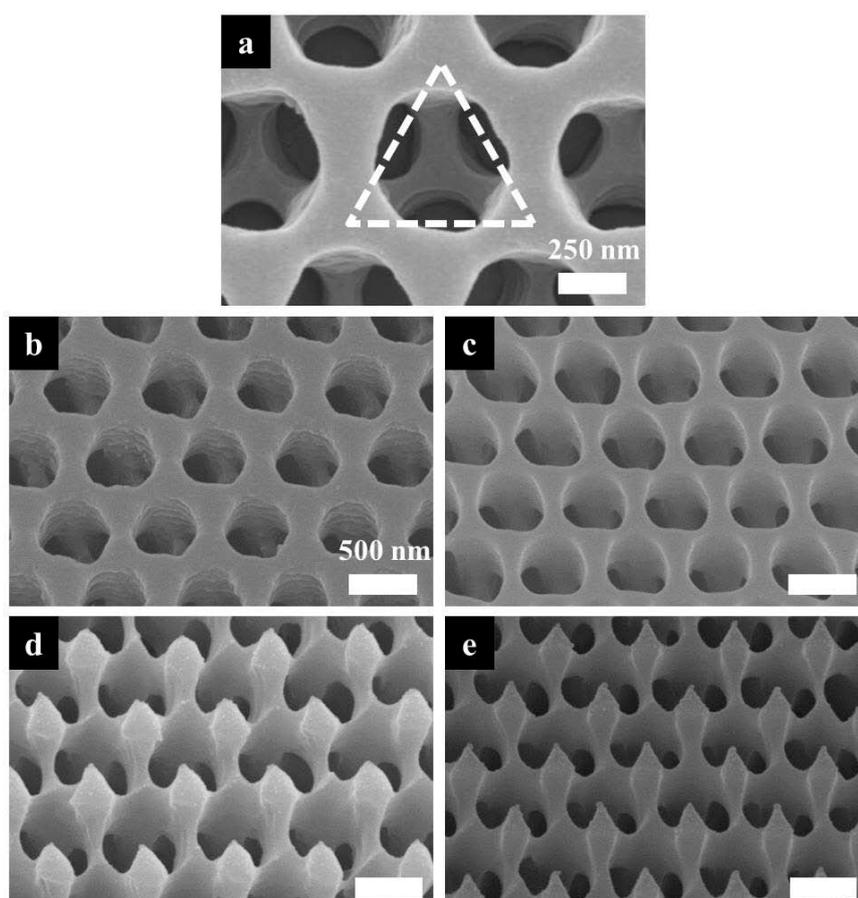
**Figure S1.** (a) SEM image of the fabricated 2-layer FCC structure showing polymeric density distribution. (b-e) 30° tilted SEM images of the feature-controlled periodic nanostructure arrays produced using FCC photonic crystals under various SF<sub>6</sub> RIE conditions, with etching durations of (b) 0 min, (c) 2 min, (d) 4 min, and (e) 6 min.
