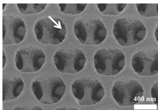
**Figure S3.** 25° tilted SEM image of the fabricated nanostructure arrays after the directional Ag-deposition step, using 2 min-etched 2-layer FCC structures.
