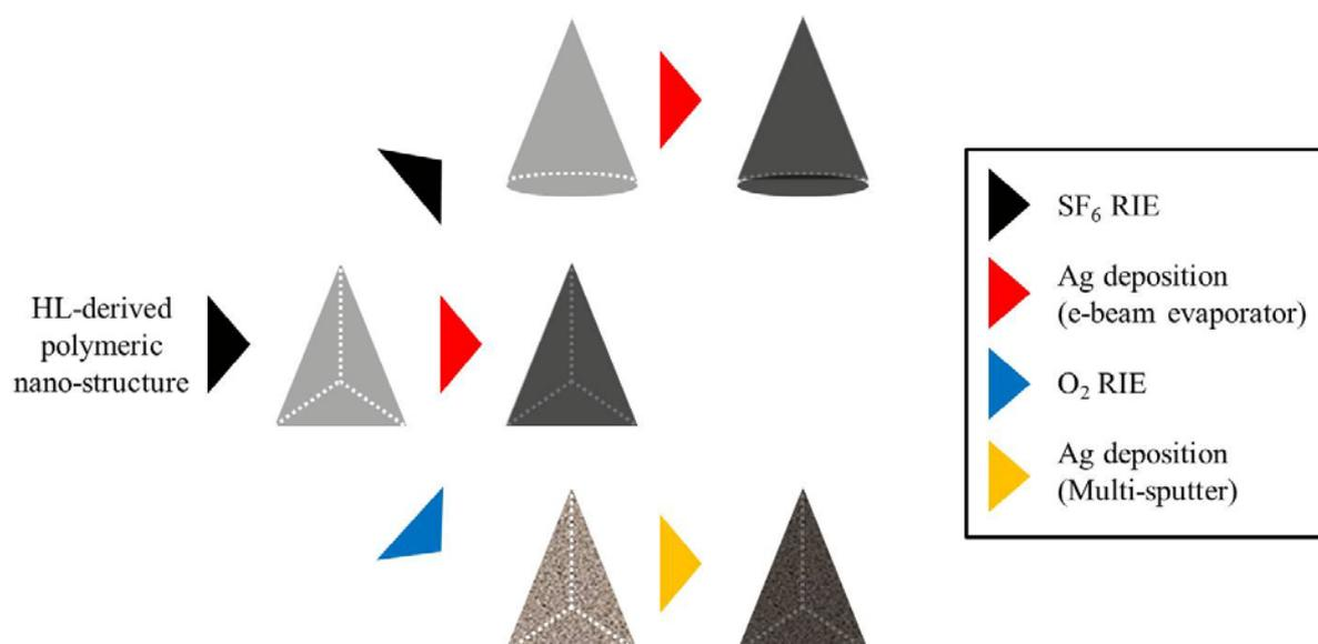
**Figure S2.** Process flow diagram for fabricating dual length-scale nanotip arrays with controllable morphological features under different fabrication conditions.
