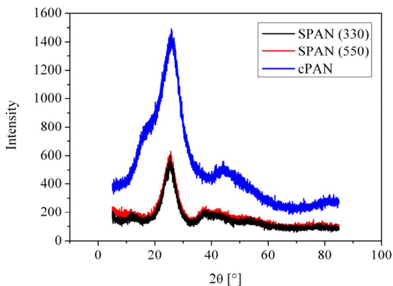
**Figure S3.** XRD patterns of cPAN (blue), SPAN<sub>330</sub> (black) and SPAN<sub>550</sub> (red).
