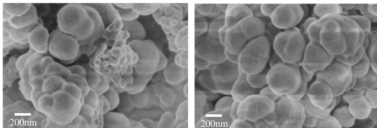
**Figure S4.** SEM images of SPAN<sub>330</sub> (left) and SPAN<sub>550</sub> (right).
