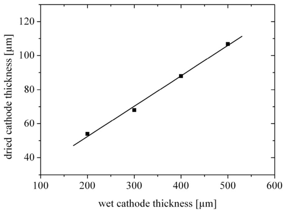
**Figure S8.** Linear dependence of the cathode thickness in the wet vs. the dried state (doctor blading).
