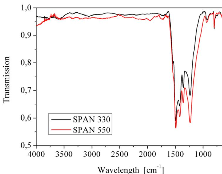
**Figure S5.** FTIR spectra of SPAN<sub>330</sub> (black) and SPAN<sub>550</sub> (red).
