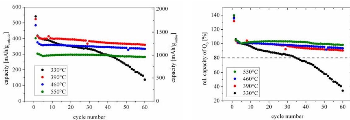
**Figure S1:** Influence of the synthesis temperature on cathode stability. a) absolute capacity b) relative capacity (% of Q<sub>5</sub>).
