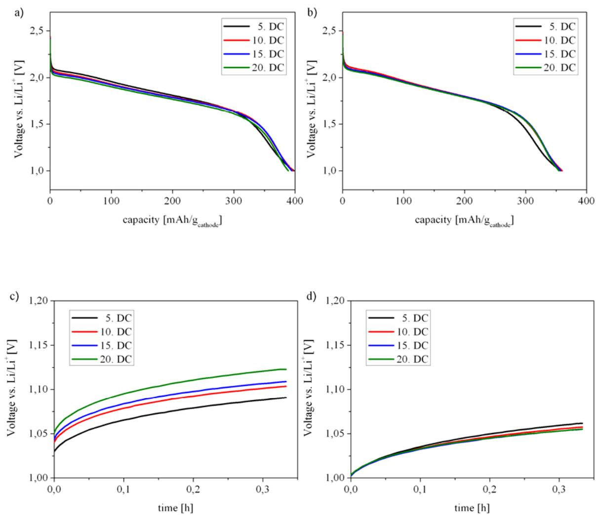
**Figure S2.** Voltage profile of the  $n^{\text{th}}$  discharge (a+b) and the following pause step (c+d) of SPAN(390°C) (a+c) and SPAN(460°C) (b+d).
