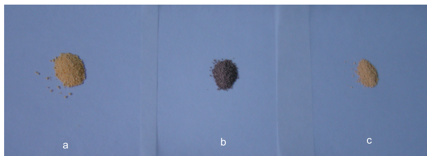
Figure S4. Photographs of (a) the \text{Bi}_2\text{O}_3/\text{Bi}_4\text{Ti}_3\text{O}_2/\text{TiO}_2 double-heterostructured prepared at 500 °C with 6:1 \text{Bi}_2\text{O}_3/\text{TiO}_2 weight ratio, (b) the above double-heterostructured nanobelt repeatedly used for four times under UV light irradiation and (c) the dark green double-heterostructured nanobelt re-annealed at 400 °C.
