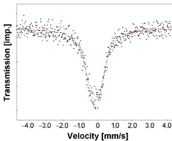
**Figure S1:**  $^{119\text{m}}\text{Sn}$  TMS spectrum of a powdered Sn doped  $\alpha\text{-Fe}_2\text{O}_3$  with doping level of 16:100.
