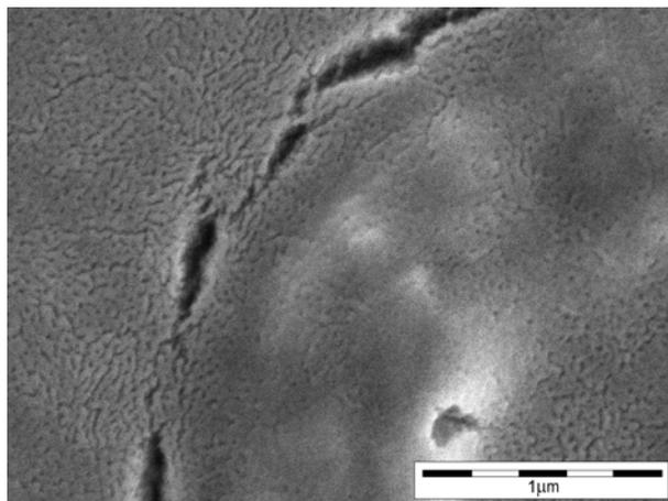
**Figure S7:** Visible cracking occurred in case of Sn-doped samples with a tin loading of 20:100.
