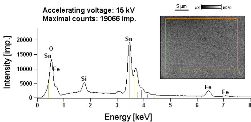
**Figure S3:** EDX of Sn-doped sample with 8:100 ratio plot showing a presence of Fe, O, Sn and Si atoms. With respect to a high penetration of X-rays, a majority of Sn and Si atoms originates from the substrate. Therefore it was not possible to observe a clear trend in growth of Sn peak intensity with increased doping fraction by EDX. The spectrum above belongs to Sn-doped sample with 8:100 ratio.
