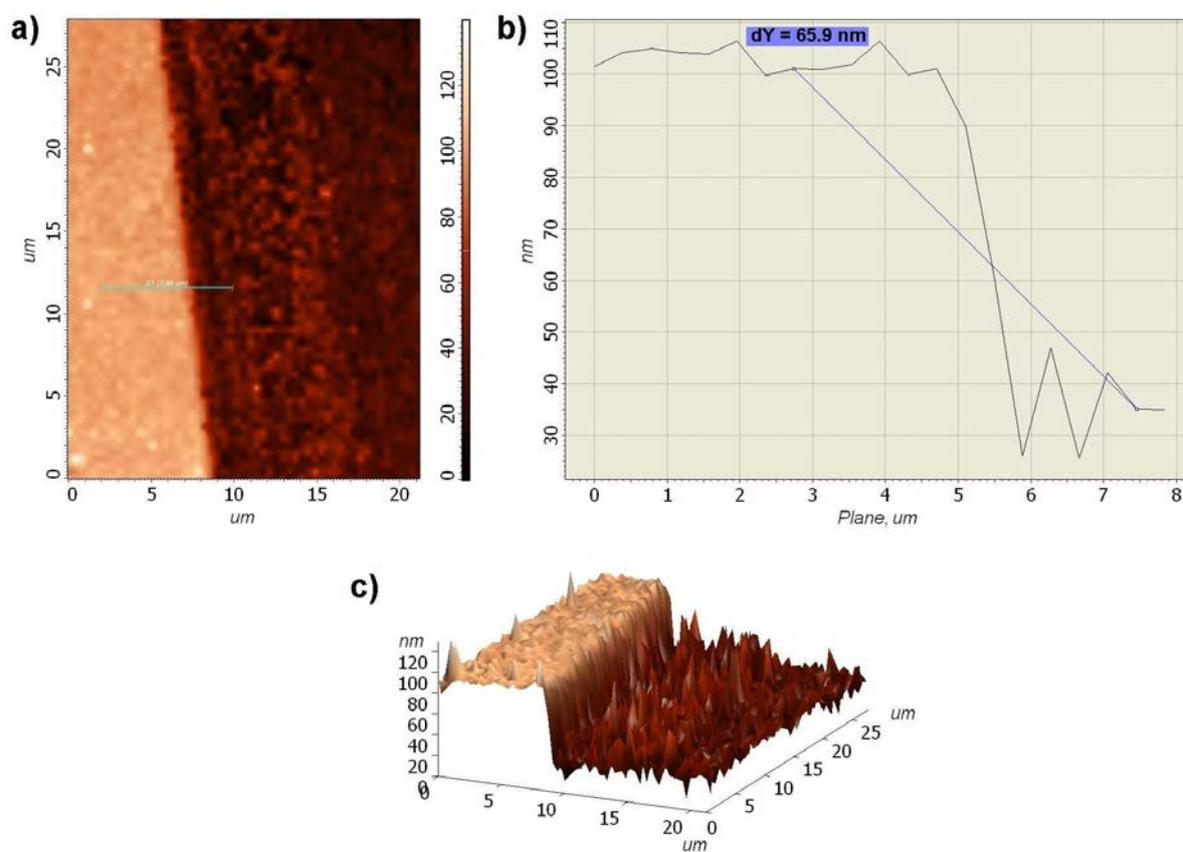
**Figure S4:** AFM 2D top view image (a) of needle scratch and its profile (b) supplemented with its 3D topography (c). This is a scan of Sn-doped hematite film (8:100). Scratch height measurement enables to estimate the overall film thickness (~65 nm). Similar results were obtained within the whole series.
