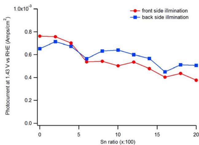
**Figure S5:** Photocurrents at 1.43 V vs. RHE versus the Sn doping (with both front and back illumination) for the series of samples treated at 800 °C.
