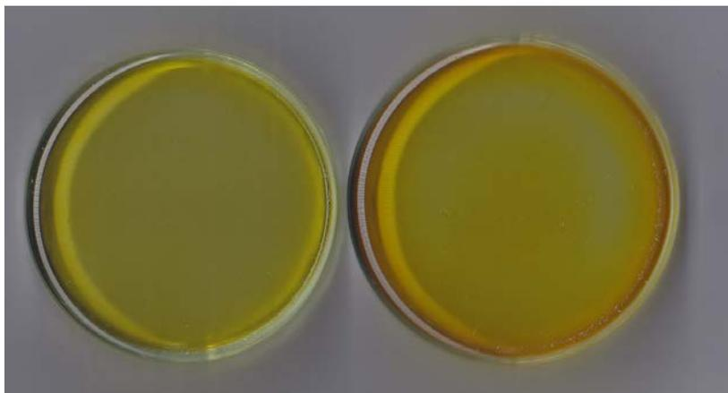
**Figure S6:** Bright solution of  $\text{FeCl}_3$  (left) gets darker after addition of  $\text{SnCl}_2$ .
