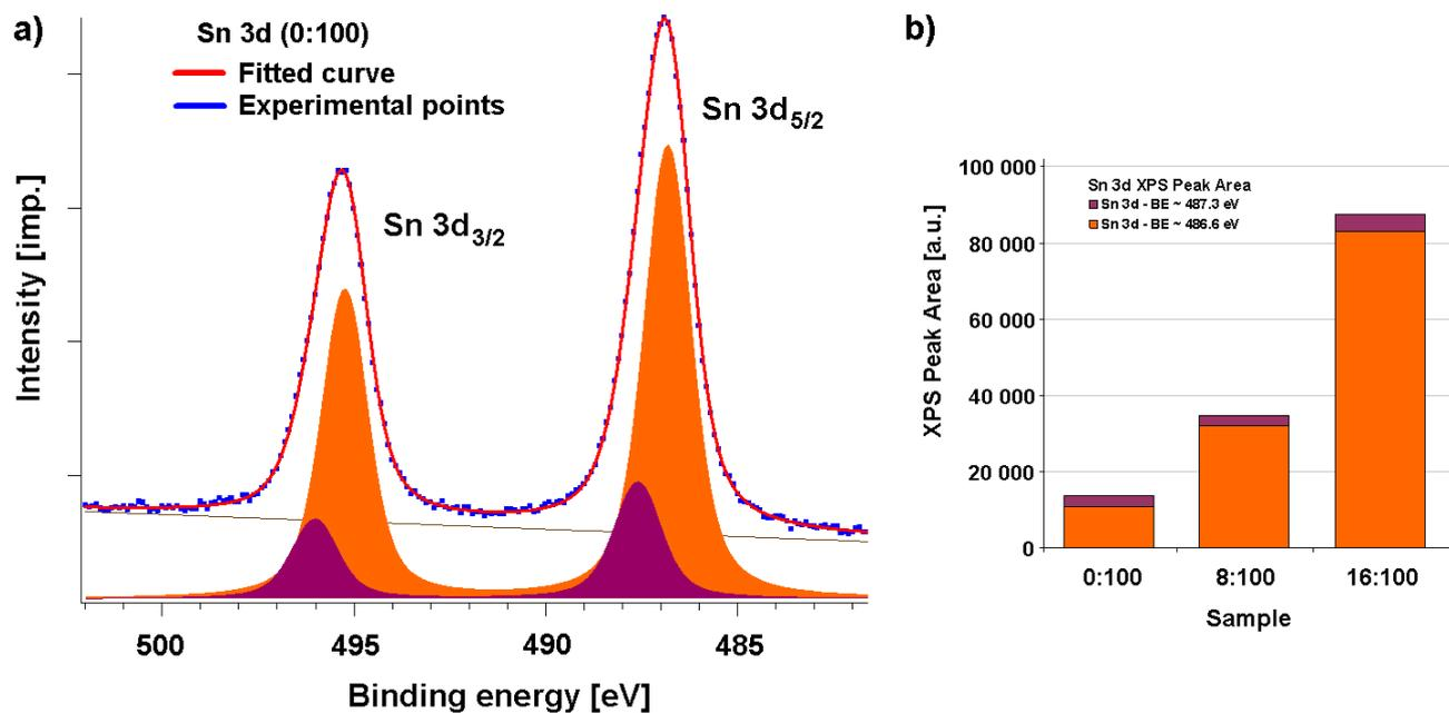
**Figure S2:** (a) Fit XPS plot of intentionally undoped sample (0:100) and (b) relative surface areas of fit Sn 3d XPS peaks. Presented XPS data are cleaned from Auger electrons and satellites. The specimens were sputtered by argon ion gun for 10 min.
