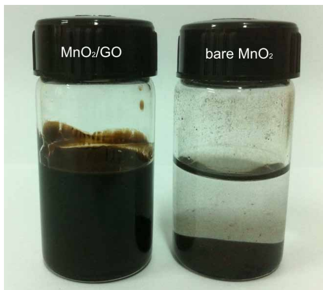
Figure S6. Digital photos of MnO 2 /GO (left) and bare MnO 2 (right) into water (0.1 g/mL). MnO 2 /GO was well dispersed in water, this can be attributed to a large amount of oxygen-containing groups existed on GO sheets. In contrast, bare MnO 2 nanocrystals have not good dispersion in water.
