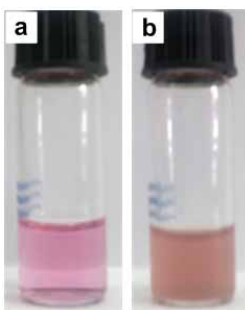
Fig. S3 Photograph of the dispersion stability of nanocarrier in a serum-containing medium.
