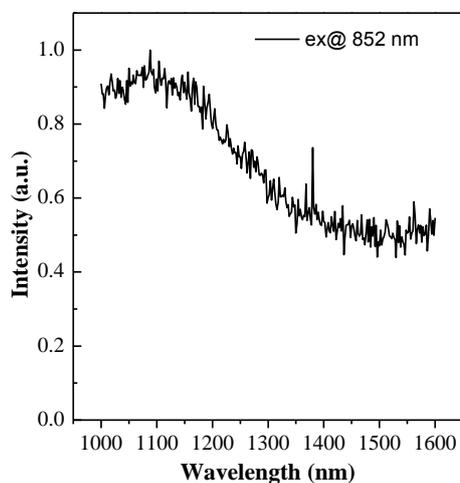
**Fig. S1** PL spectrum Te<sub>4</sub>(Ga<sub>2</sub>Cl<sub>7</sub>)<sub>2</sub> sample under the excitation of 852 nm.
