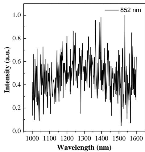
**Fig. S2** PL spectrum  $\text{Te}_4(\text{Al}_2\text{Cl}_7)_2$  sample under the excitation of 852 nm.
