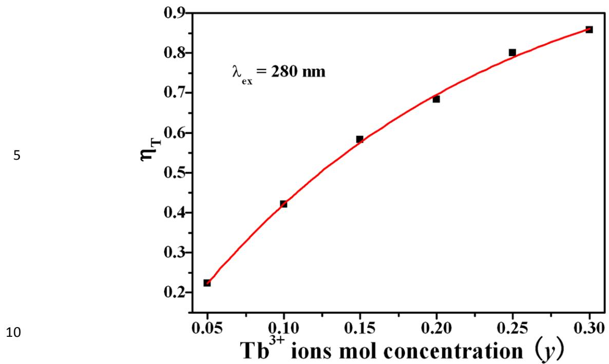
**Fig. S5** Energy transfer efficiency from  $Ce^{3+}$  to  $Tb^{3+}$  in KCG:  $Ce^{3+}, yTb^{3+}$  samples ( $\lambda_{ex} = 280 \text{ nm}$ ).
