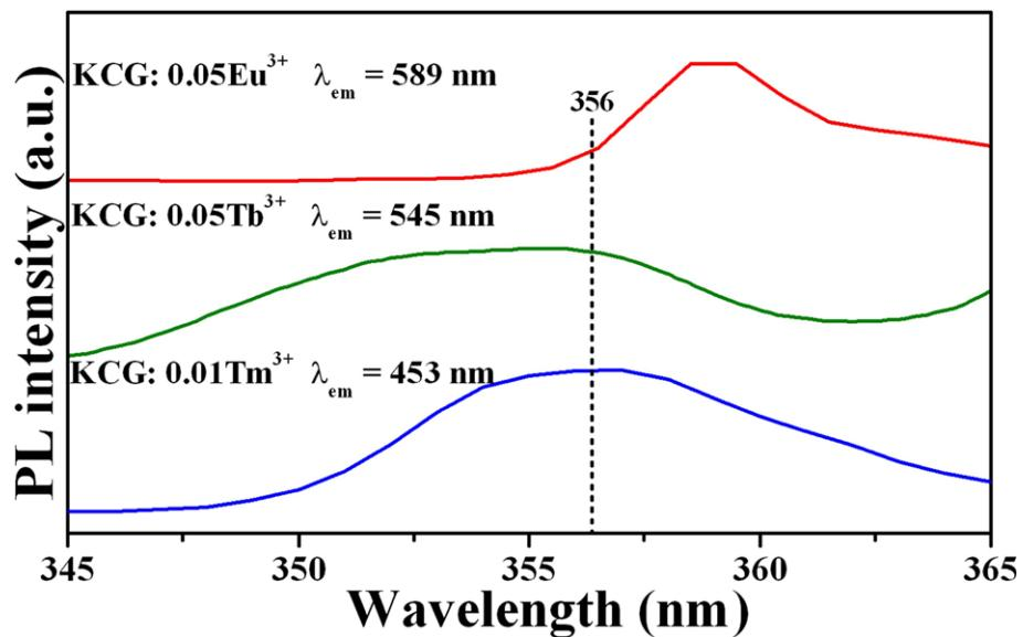
**Fig. S2** The excitation spectra of KCG: Eu<sup>3+</sup>/Tb<sup>3+</sup>/Tm<sup>3+</sup> phosphors monitoring with the characteristic emission of Eu<sup>3+</sup>/Tb<sup>3+</sup>/Tm<sup>3+</sup>.
