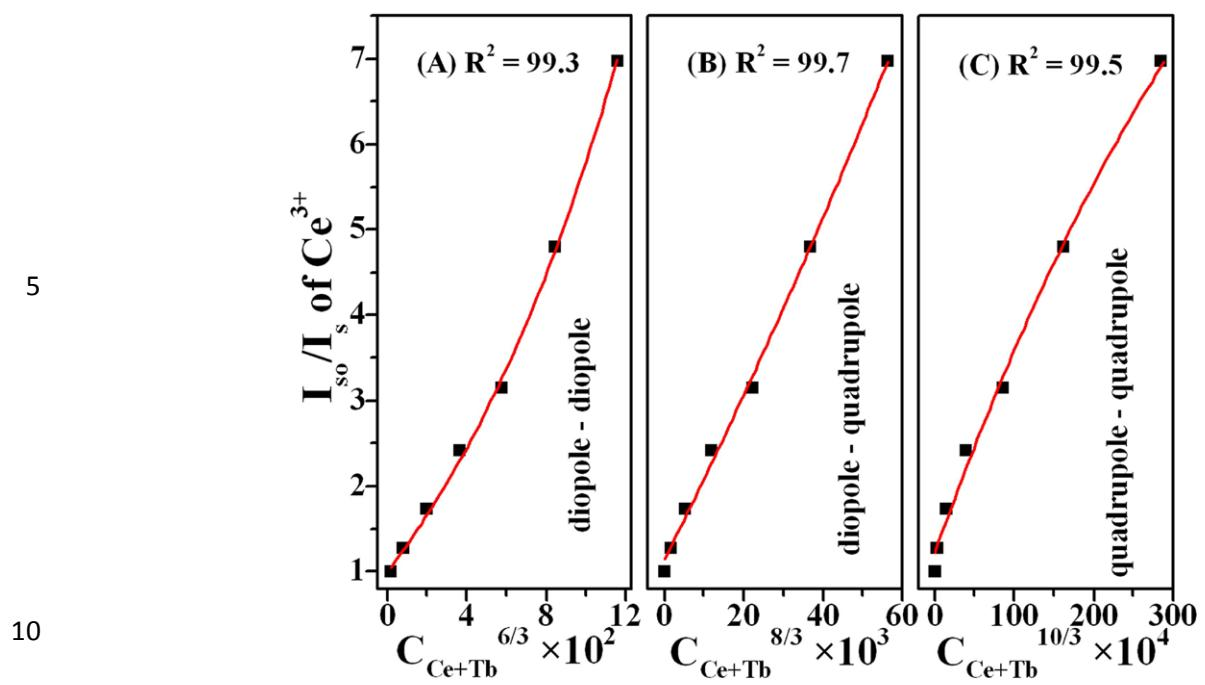
**Fig. S6** Dependence of  $I_{so}/I_s$  of  $\text{Ce}^{3+}$  on (A)  $C_{\text{Ce}+\text{Tb}}^{6/3}$  (B)  $C_{\text{Ce}+\text{Tb}}^{8/3}$  (C)  $C_{\text{Ce}+\text{Tb}}^{10/3}$ .
