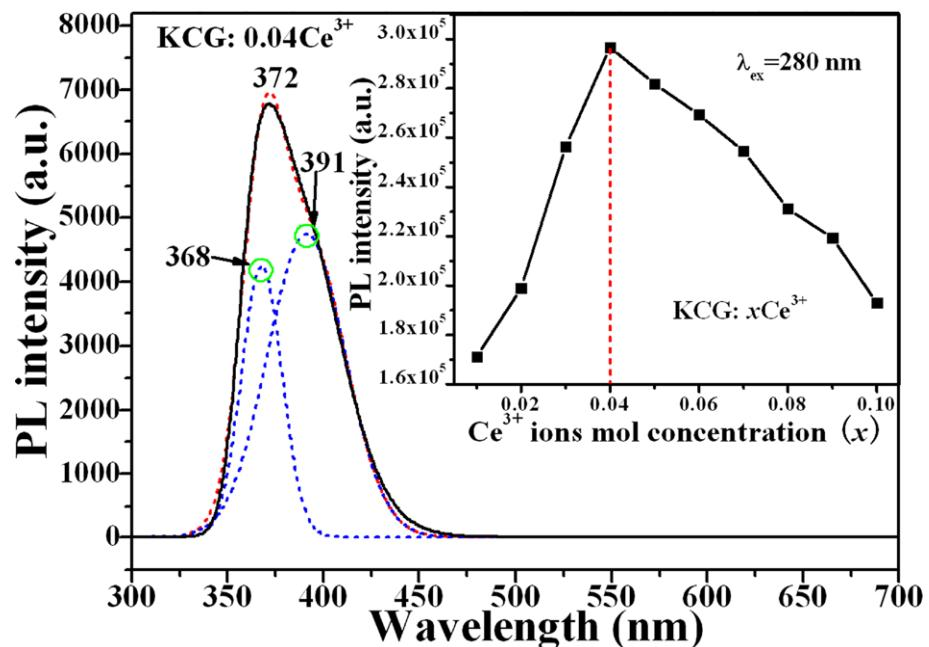
**Fig. S3** The emission spectra of KCG: 0.04 $\text{Ce}^{3+}$  sample ( $\lambda_{\text{ex}} = 280$  nm) and the deconvoluted emission spectrum of the emission band as a sum of two Gaussian bands. The inset shows the PL intensity of KCG:  $x\text{Ce}^{3+}$  samples as a function of  $\text{Ce}^{3+}$  doping concentration under the excitation of 280 nm UV.
