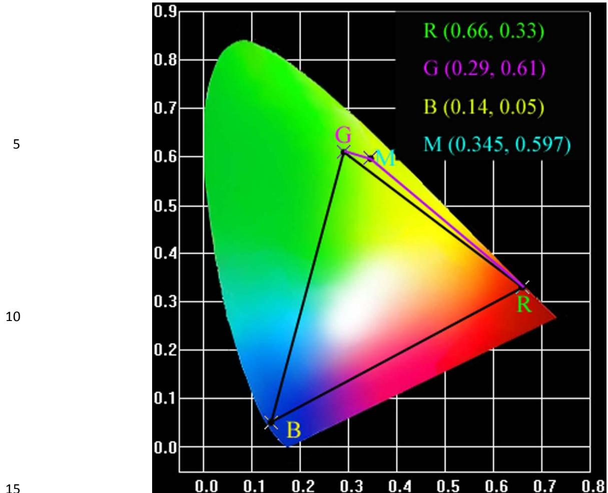
**Fig. S8** CIE chromaticity diagram of standard FED phosphors and KCG:  $0.12\text{Mn}^{2+}$  sample. R, G, B and M represent the CIE Chromaticity coordinates of  $\text{Y}_2\text{O}_2\text{S}:\text{Eu}^{3+}$  (P22R),  $\text{ZnS}:\text{Cu}:\text{Au}:\text{Al}$  (P22G),  $\text{ZnS}:\text{Ag}:\text{Cl}$  (P22B) and KCG:  $0.12\text{Mn}^{2+}$  phosphors, respectively.
