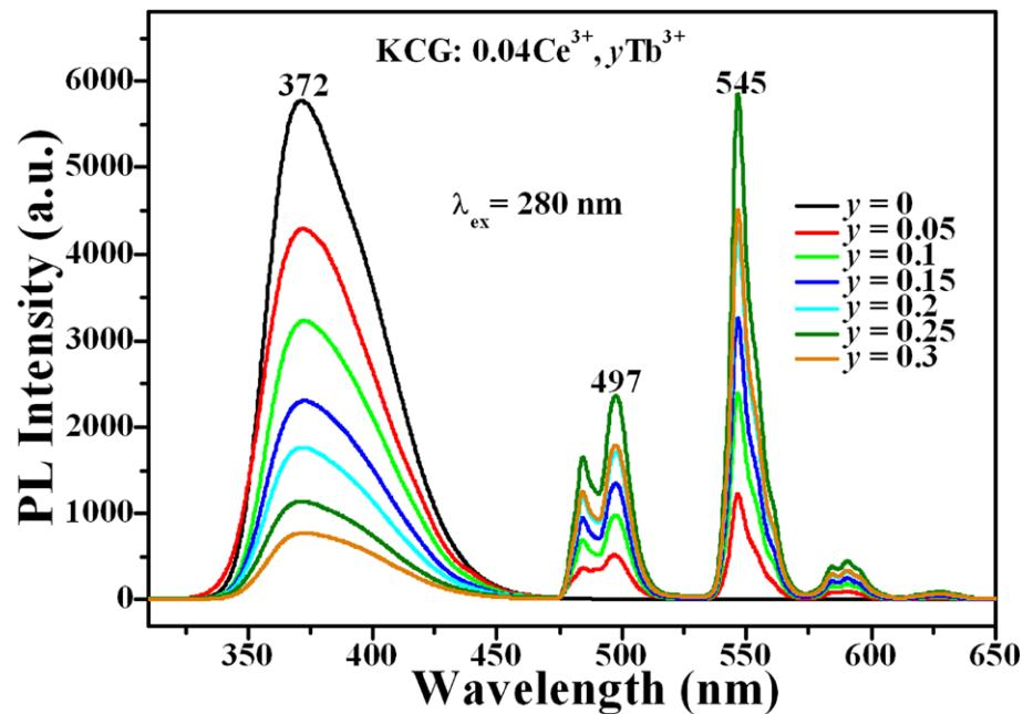
**Fig. S4** The variation of PL spectra of KCG: 0.04Ce<sup>3+</sup>, yTb<sup>3+</sup> samples with changing Tb<sup>3+</sup> and fixed Ce<sup>3+</sup>.
