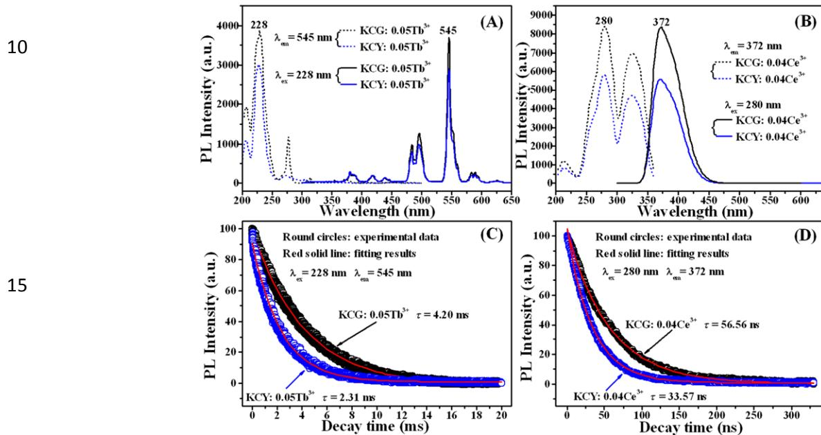
**Fig. S1** PL excitation and emission spectra (A and B) along with the decay curves and lifetimes (C and D) of  $\text{Tb}^{3+}/\text{Ce}^{3+}$  in KCG and KY host.
