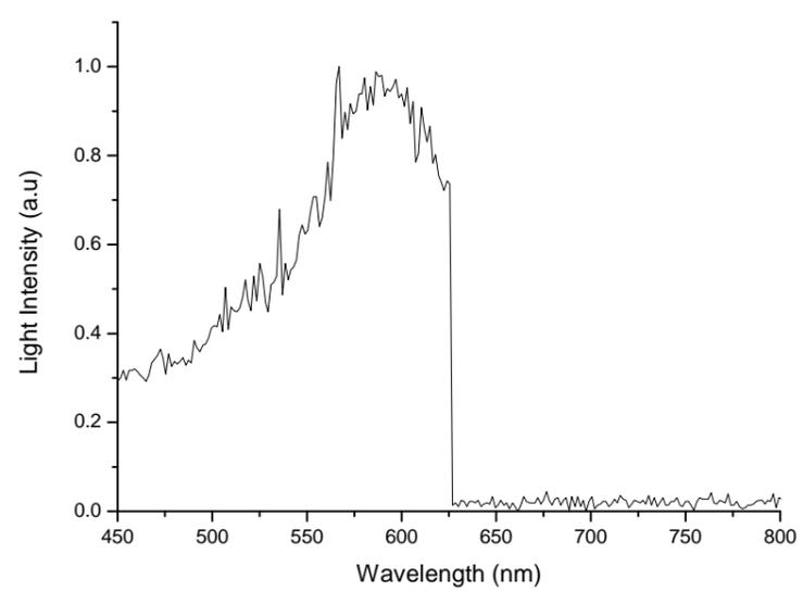
**Figure S4.** – Electroluminescence spectrum of working OLED device, with turnoff at 625 nm.
