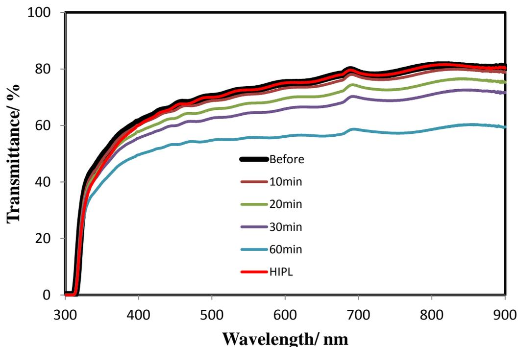
**Figure S2.** Transmittance spectra of PET films before and after HIPL sintering, and heated at 200 °C with different times (air as a reference).
