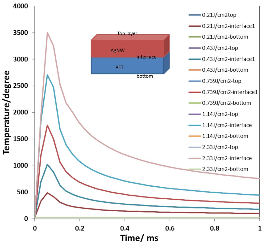
**Figure S3.** Simulated temperature change in the dense Ag film and at the interface with various light intensity.
