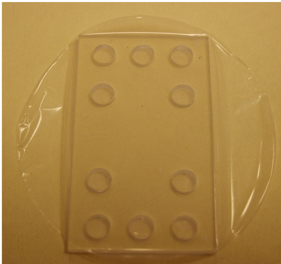
ESI – Fig 1. Photograph of a polycarbonate nanocapillary array membrane (NCAM) after bonding to a device stack. The circular NCAM is then trimmed with a razor blade along the rectangular device edge before bonding another poly (methylmethacrylate) (PMMA) microfluidic channel layer to the exposed side.
