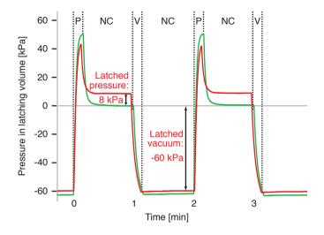
Supplementary data. Pressure measured inside the latching volume while actuating a V-latching (green) and PV-latching (red) valve with 10 s pressure (P) or vacuum (V) pulses (NC = no connection to valve). While both valves latch open in a similar fashion, only the PV-latching valve traps 8 kPa pressure in the latching volume to hold the valve closed against pressures in the fluidic system.
