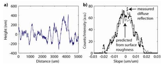
**Fig. 2** a) Trace of the height versus distance taken with a Dektak Surface Profilometer. b) Comparison between slope distributions of a milled flat surface measured by reflected intensity and surface profilometry. Both measurements yield similar distributions, indicating specular scattering behavior due to surface roughness.
