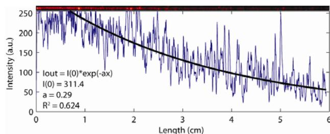
**Fig. 1** An image of the perpendicularly scattered light and a single exponential fit to the intensity versus distance. The 90  $\mu\text{m}$  x 90  $\mu\text{m}$  waveguide measures a loss of 0.29  $\text{cm}^{-1}$  or 1.26 dB/cm at 632 nm.
