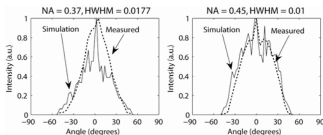
**Fig. 3** Measured and simulated intensity versus angle plots are shown for 1 mm x 1 mm waveguides of varying roughness. Gaussians fits to the measured roughness with a HWHM of (Left) 0.0177 and (Right) 0.01 are used to perform Monte Carlo ray tracing simulations.
