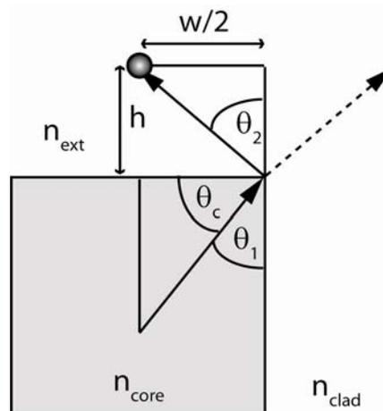
**Fig. 1** Ray tracing approach to determining the maximum waveguide width necessary to collect a point source emission located a distance  $h$  away from the waveguide face.
