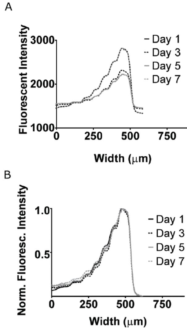
Sup. Fig. 1 Experimental determination of gradient degradation over time. Represented are the profiles of a gradient taken every other day. The device was kept in a cell incubator at 37 C. Panel A shows raw fluorescence intensity values while panel B shows normalized values.
