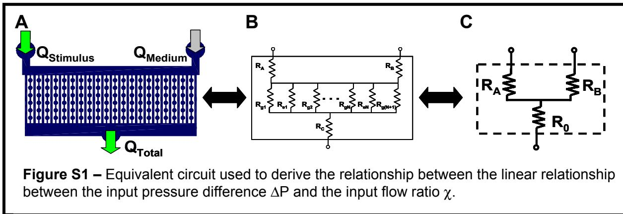
**Figure S1** – Equivalent circuit used to derive the relationship between the linear relationship between the input pressure difference  $\Delta P$  and the input flow ratio  $\chi$ .
