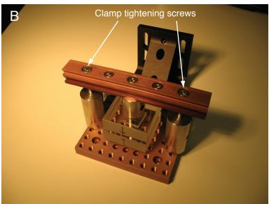
Assembled bonding clamp. When the outermost 1/4-20 screws on the beam are tightened, the bonding stack is compressed between a 14 mm diameter flat screw in the base (visible in Photo A) and a 25 mm diameter by 25 mm tall post attached to the cross beam.
