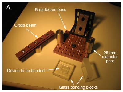
Disassembled bonding clamp, showing an assembled glass-Teflon-glass device on top of a borosilicate glass bonding block (McMaster-Carr part 8476K127). The clamp is constructed from optical hardware (Thorlabs), including an 11 cm square aluminum breadboard base, two 25 mm diameter by 50 mm tall threaded posts, and a 15 cm long cross beam.
