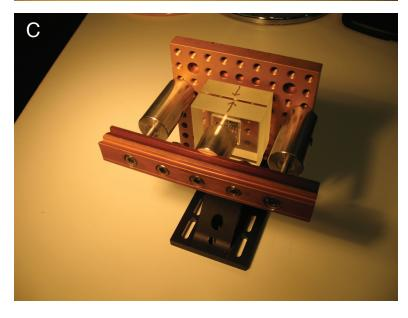
Assembled bonding clamp turned on its side and ready to be placed in oven.
