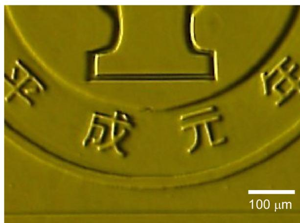
**Figure S2.** Microstructure on the pSPNIPAAm hydrogel sheet formed by micropatterned light irradiation through x10 objective lens.
