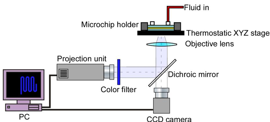
**Figure S1.** Computer-controllable maskless micropattern projection unit mounted on a microscope.
