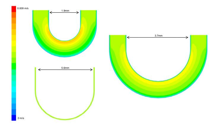
(Channel Width: 1 mm; shear stress: 2.9 dyn/cm<sup>2</sup> for all three simulations)
