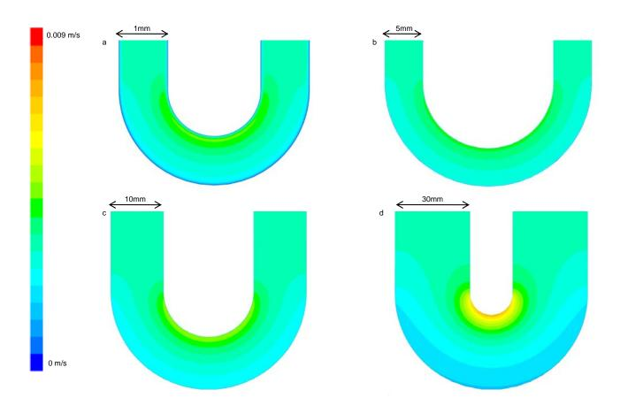
(Gap spacing: 1.9 mm; shear stress: 1.9 dyn/cm<sup>2</sup> for all four simulations)
