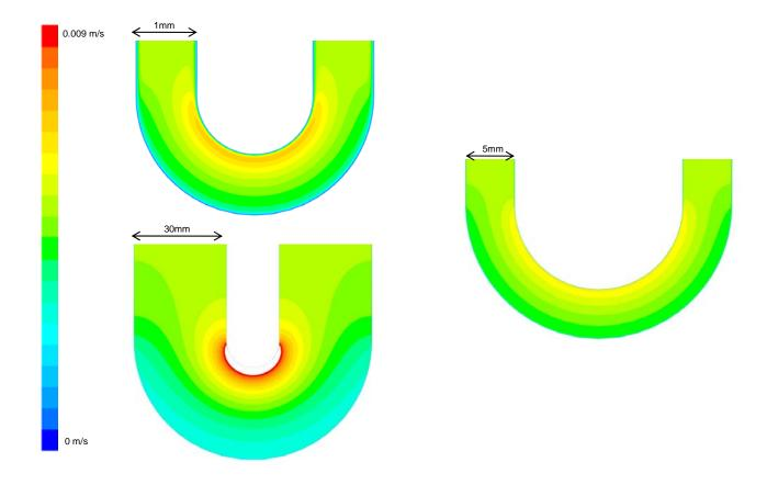
(Gap spacing: 1.9 mm; shear stress: 2.9 dyn/cm<sup>2</sup> for all three simulations)
