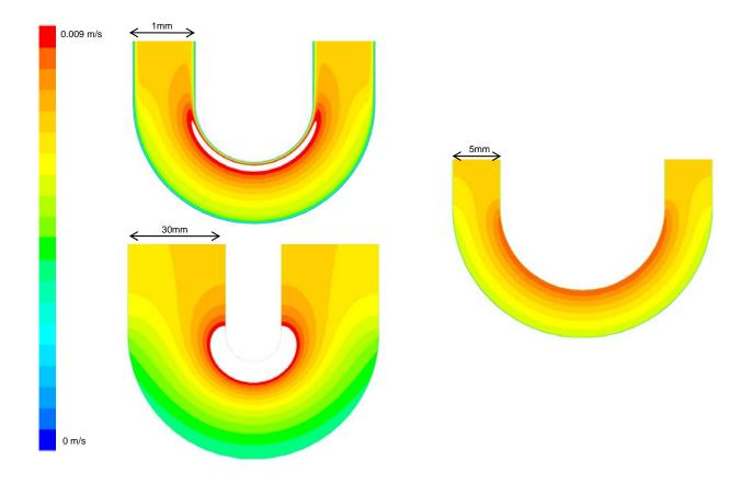
(Gap spacing: 1.9 mm; shear stress: 3.9 dyn/cm<sup>2</sup> for all three simulations)
