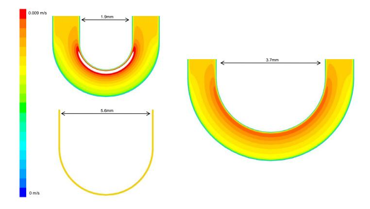
(Channel Width: 1 mm; shear stress: 3.9 dyn/cm<sup>2</sup> for all three simulations)
