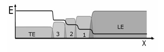
Figure A1. Schematic of the plateau shaped zones between LE and TE zones in ITP under steady state conditions. The electric field profile is overlaid on the concentration profile in each ITP zone.
