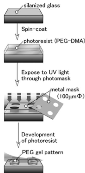
**Fig. S3** Process flow for the fabrication of PEG hydrogel microstructures by photolithography technique.
