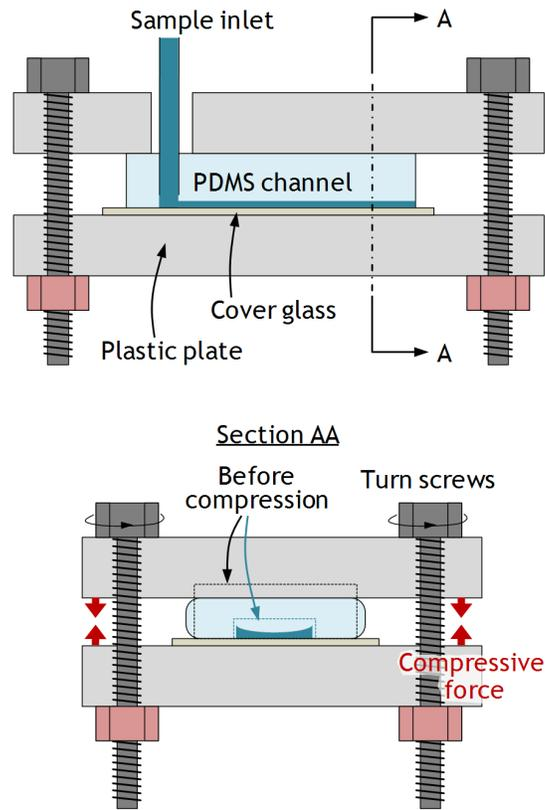
**Fig. S2.** Compression system with bolts and nuts to adjust the channel height. The elastomeric microfluidic device is compressed to change the cross-sectional size of the channel by fastening the bolts.
